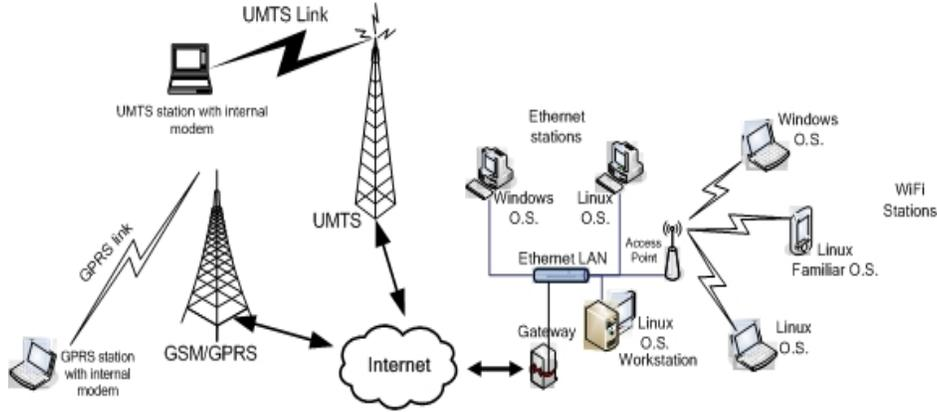
Figure 1: The Experimental Test-bed Infrastructure: Real Network
