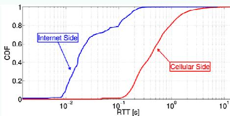
it is important to take into the proper account the presence of such device when performing network measurements: it can be useful for those interested in estimating the performance as seen by the users - in fact, they only see the cellular side - while being an issue for those interested in looking at the end-to-end performance.
