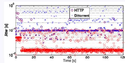
The throughput of the HTTP-like flow is higher with respect to the other flow, their average values being 350Kbps and 58Kbps respectively. Also, the jitter of the two flows achieve different values over time. The average value for the HTTP-like is 32ms, while for the Bittorrent-like flow is 191ms. This is the effect of a PCMS.
