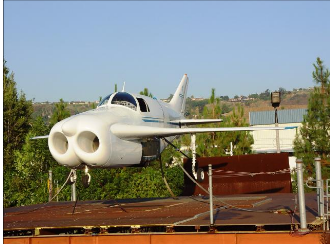
Figure 6. duPont Aerospace DP-1 in a tethered hover test. (Courtesy of duPont Aerospace Company)
