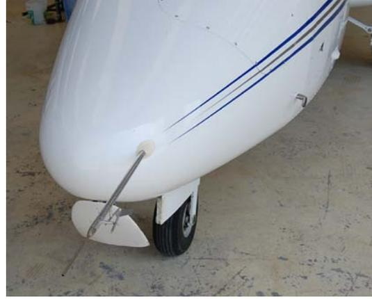
Figure 7. Pitot probe with  $\alpha$ - and  $\beta$ -flags.
