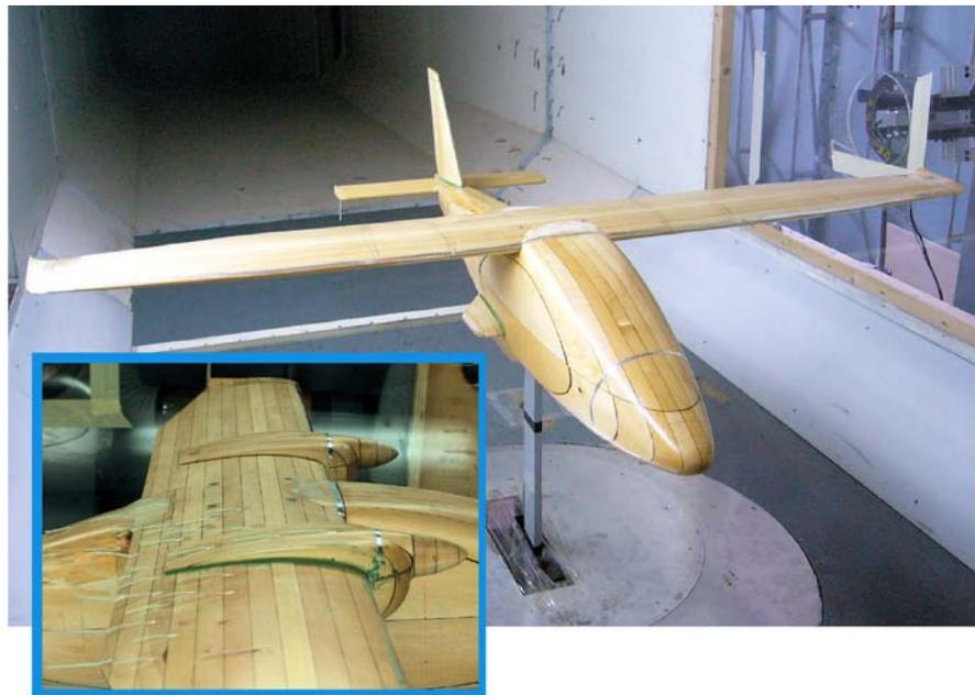
**Figure 3 Scaled model of P2006T in the low-speed wind tunnel of the University of Naples “Federico II”.**
