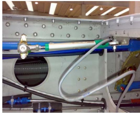
Figure 9. Position transducer – Aileron control
