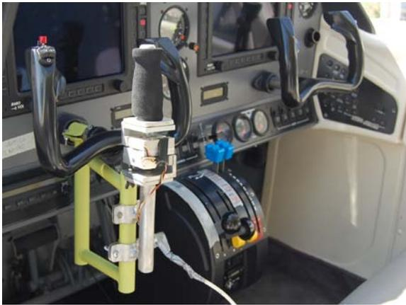
Figure 8. Load cells for stick force measurements.
