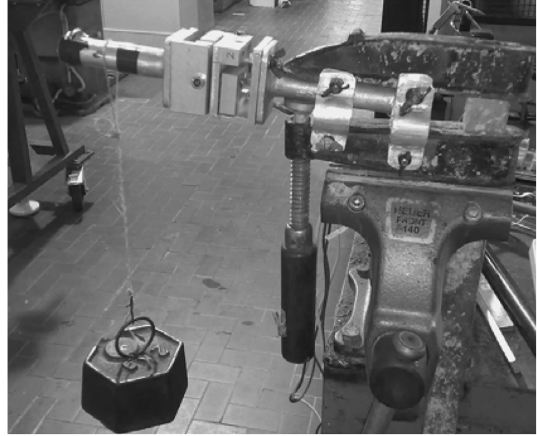
Fig. 10 Load cells calibration.
