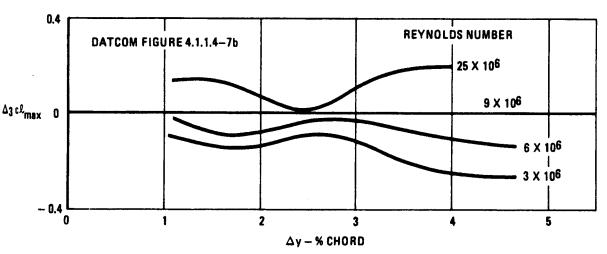
FIGURE B-6 EFFECT OF REYNOLDS NUMBER ON SECTION MAXIMUM LIFT
