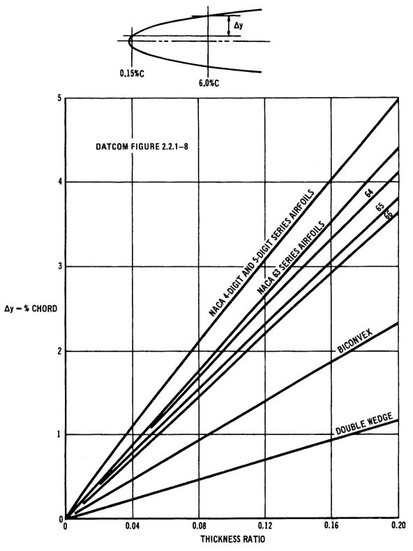
FIGURE B-2 VARIATION OF LEADING-EDGE SHARPNESS PARAMETER WITH AIRFOIL THICKNESS RATIO
