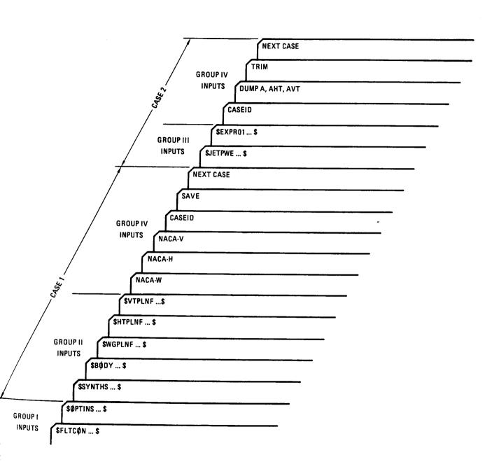
FIGURE 24 TYPICAL "STACKED CASE" SETUP
