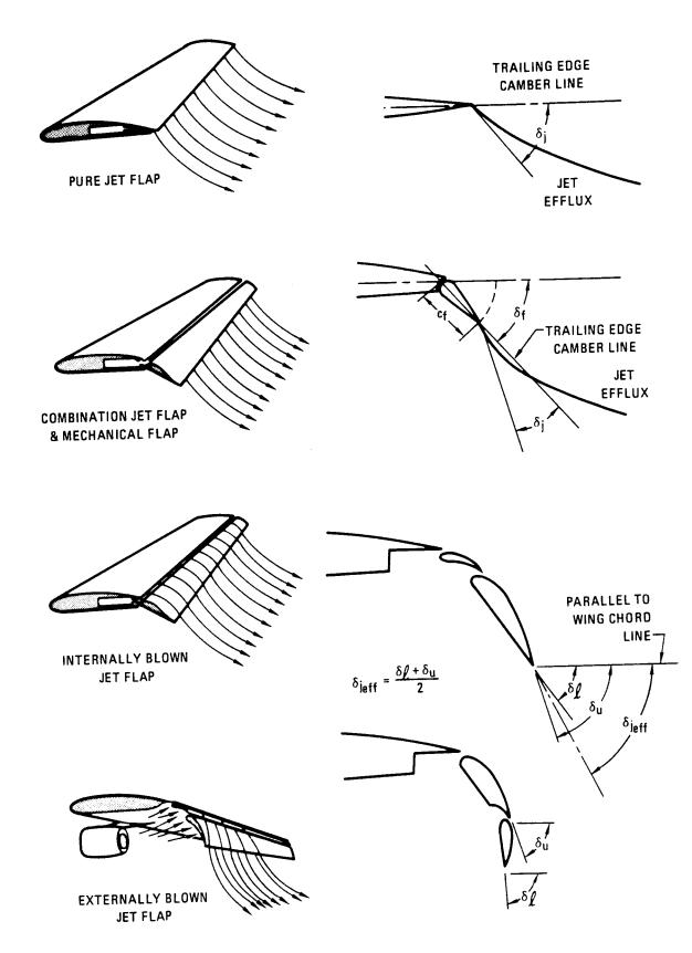
FIGURE 18 JET FLAP INPUT DEFINITIONS
