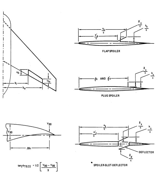
FIGURE 19 INPUT FOR NAMELIST ASYFLP - ASYMMETRICAL CONTROL DEFLECTION INPUT
