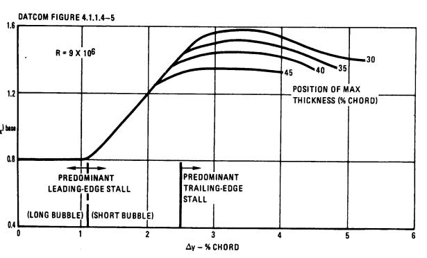
FIGURE B-3 AIRFOIL SECTION MAXIMUM LIFT COEFFICIENT OF UNCAMBERED AIRFOILS
