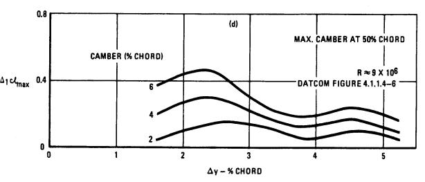
FIGURE B-4 EFFECT OF AIRFOIL CAMBER LOCATION AND AMOUNT ON SECTION MAXIMUM LIFT (CONCLUDED)
