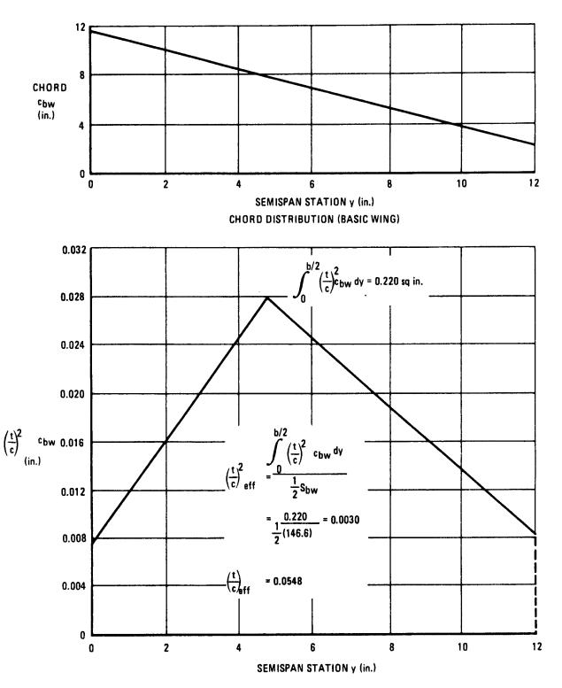
FIGURE B-9 GRAPHICAL SOLUTION FOR (t/c) EFFECTIVE (CONCLUDED)
