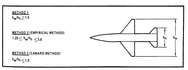
METHOD IN RANGE 1.0  $\leq$   $b_{\text{W}}/b_{\text{h}}$   $\leq$  1.5 can be selected using variable "DWASH" in Namelist WGSCHR
