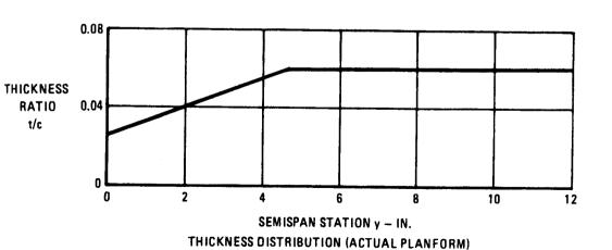
FIGURE B-9 GRAPHICAL SOLUTION FOR (t/c)effective
