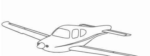
(c) wing-body-horizontal tail (WBH)
