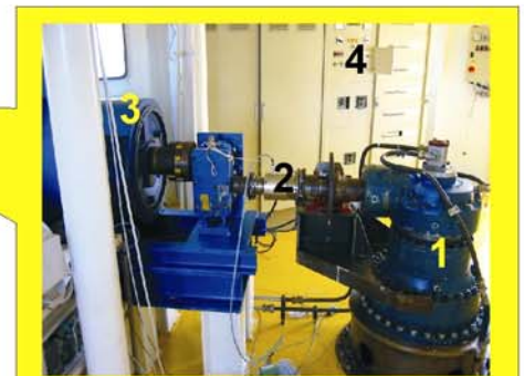
Buoy inside: multiplier (1), torque-meter (2), electric generator (3), control panel (4)
