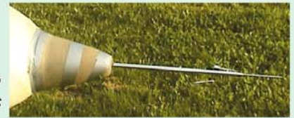
Pitot Probe with angle indicators
