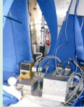
Acquisition System, Radio Modem and GPS
