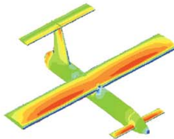
3D Pressure coefficient distributions (panel methods)
