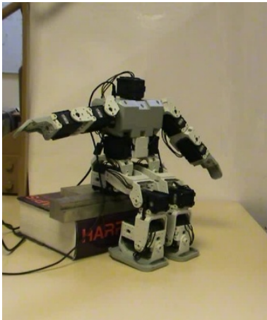
Fig. 1. A picture of the Bioloid assembled as a humanoid robot
