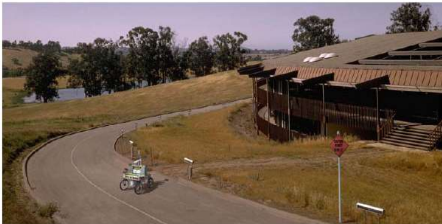
Stanford AI Laboratory / CMU (Moravec) drove the Cart through several 20-m courses (each taking about 5 h)
