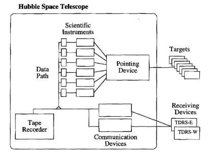
The pointing subsystem is responsible for orienting HST toward a target and locking it at the center of the field of view of the instrument.
