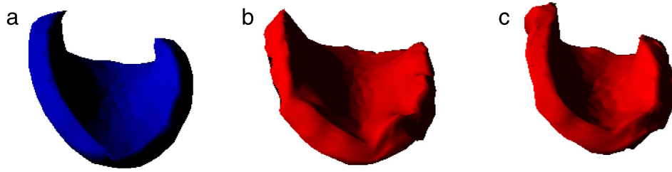
Fig. 9. Deformations on the generated sequence (a), on the tracked mesh with the standard FEM (b), and with the co-rotational FEM (c).
