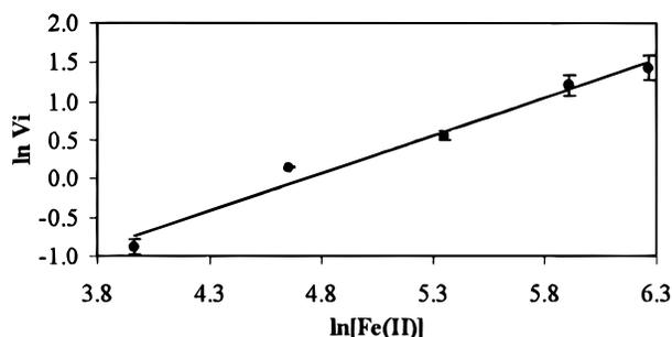
**Figure 4.** Logarithmic plot of initial rates of dopamine oxidation ( $\mu\text{M s}^{-1}$ ) vs  $\text{Fe}^{2+}$  concentration,  $r^2 = 0.98$ . Dopamine was oxidized as detailed in Figure 1. Initial rates of dopamine oxidation were determined after 1 min. Slope =  $1.05 \pm 0.05$ .
