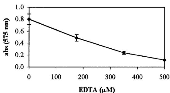
**Figure 7.** Plot of the absorbance at 575 nm of the dopamine–Fe(III) chelate vs EDTA concentration in 0.1 M Tris buffer, pH 7.4. Dopamine and Fe<sup>3+</sup> concentration were 500 and 350  $\mu\text{M}$ .
