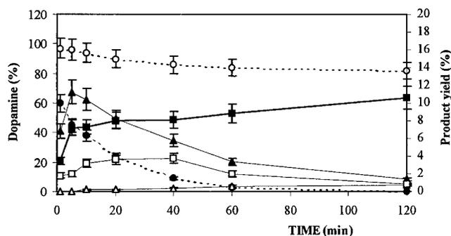
**Figure 2.** Time course of dopamine oxidation (dashed lines, left axis) and percent product yields (right axis) by oxidation of 500  $\mu$ M dopamine with 350  $\mu$ M ferrous ions in the presence and in the absence of 5 mM linoleic acid 13-hydroperoxide. Dopamine decay: (●) with hydroperoxide; (○) without hydroperoxide. Formation of **2**: (▲) with hydroperoxide; (△) without hydroperoxide. Aminochrome formation: (■) with hydroperoxide; (□) without hydroperoxide.
