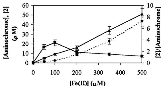
**Figure 5.** Plots of **2** (▲) and aminochrome (■) concentration (left axis) and **2**/aminochrome ratio (dashed line, right axis) against  $\text{Fe}^{2+}$  concentration.
