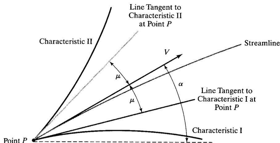
Figure 14.5 Geometry of Characteristics at a Point
