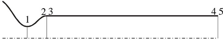
$$L_{34} := 1.5 \cdot \text{m} \quad \text{RF}_{34} := 4 \cdot f \cdot \frac{L_{34}}{D} \quad \text{RF}_{34} = 0.177 \quad p_{02} := p_0$$
