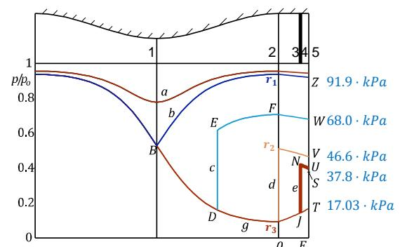
$$F_3^* = 0.1610 \xrightarrow{\substack{\text{FF} \\ (M > 1)}} M_3 = 1.569 \xrightarrow{\text{NSW}} M_4 = 0.678 \xrightarrow{\text{FF}} F_4^* = 0.254$$
