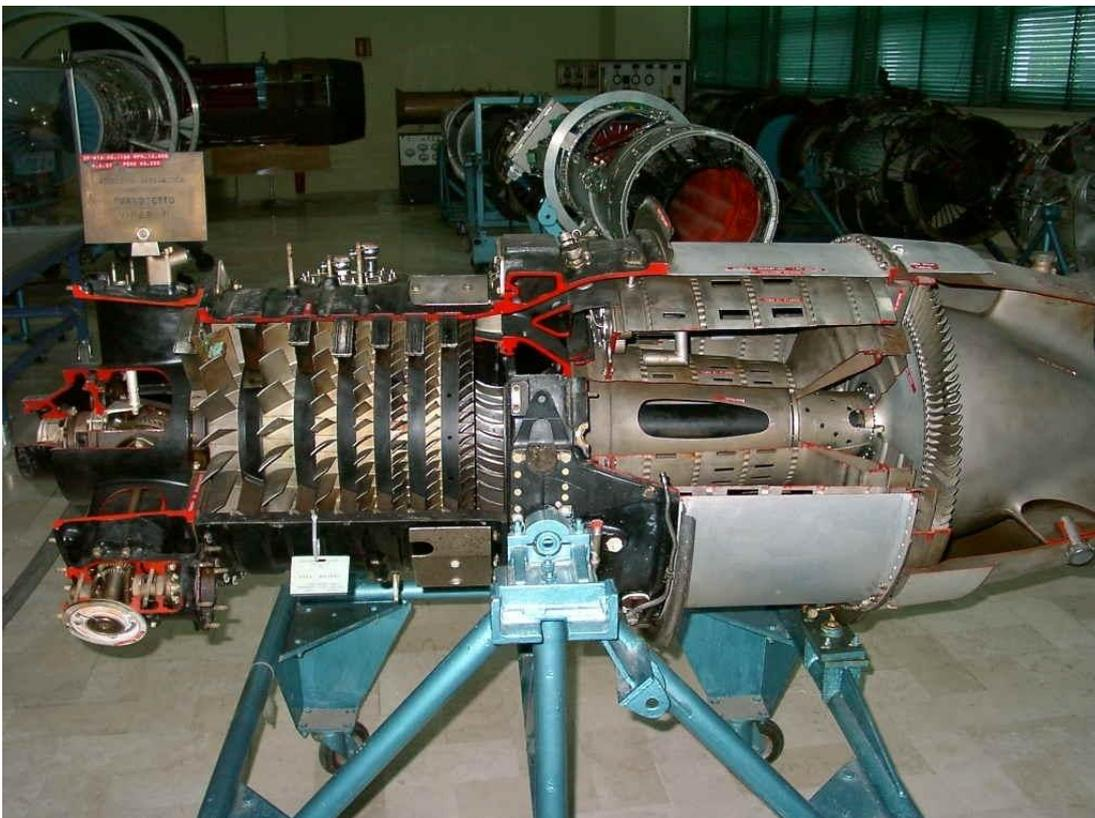
Armstrong Siddeley RR VIPER (Aermacchi MB 326). Peso 249kg,  $L=1.63m$ ,  $D=.62m$ ,  $F_{max}=12kN$ ,  $\dot{m}_a=20kg/s$ ,  $\pi_c=4.3$ , Comp 7, Turb 1.
