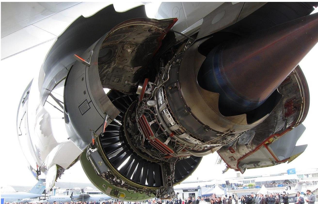
GEEnX (787, 747). Peso 6150kg,  $L=4.7m$ ,  $D=2.82m$ ,  $F_{max}=330kN$ ,  $\dot{m}_a=1200kg/s$ ,  $\alpha=9.1$ ,  $\pi_c=46$ , Comp 1/4/10, Turb 2/7.
