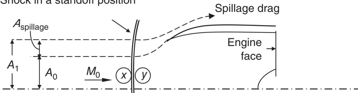
(a) Normal shock inlet in *subcritical mode* (high backpressure—low  $m$  and  $m_{cor}$ )
