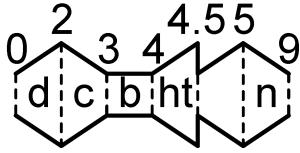
$$\alpha_p = \frac{\mathcal{P}_{i,LPT}}{\mathcal{P}_{i,tot}} = \frac{\mathcal{P}_{LPT}}{\mathcal{P}_{i,tot}} = \frac{h_{t45} - h_{t5s}}{h_{t45} - h_{9s}} \quad \tau_{tL} = \frac{h_{t5}}{h_{t45}} \quad \eta_{tL} = \frac{h_{t45} - h_{t5}}{h_{t45} - h_{t5s}} \quad \eta_{tL}\alpha_p = \frac{h_{t45} - h_{t5}}{h_{t45} - h_{9s}}$$
