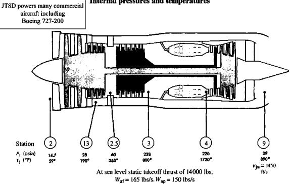
A mixed exhaust turbofan engine (JT8D from Pratt and Whitney, 1974) is described by its internal pressures and temperature, as well as air mass flow rates and the mixed jet (exhaust) velocity. Let us examine a few parameters for this engine, for a ballpark approximation.
