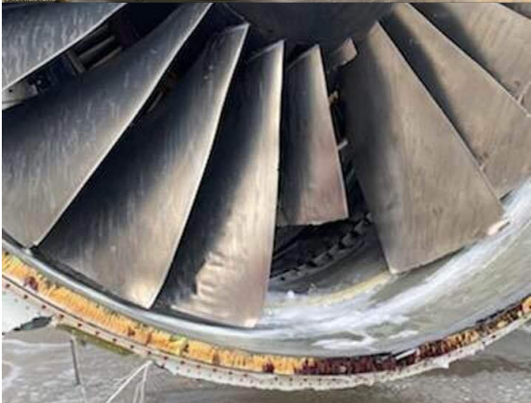
PW 4000 (777). Peso 7000kg, L=4.8m , D=2.84m , F_{max}=420kN , \alpha=6 , \pi_c=50 , Comp 1/7/11, Turb 2/7. Incidente del 20.2.2021
