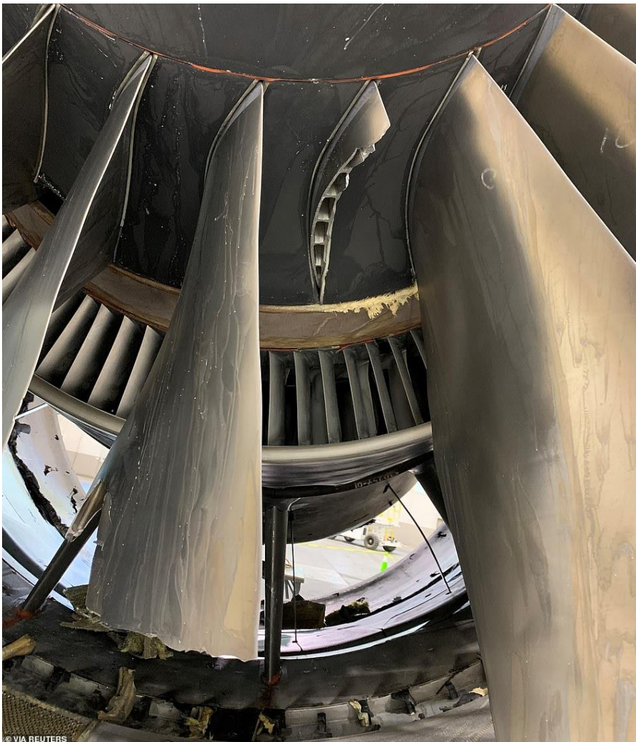
PW 4000 (777). Peso 7000kg, L=4.8m , D=2.84m , F_{max}=420kN , \alpha=6 , \pi_c=50 , Comp 1/7/11, Turb 2/7. Incidente del 20.2.2021
