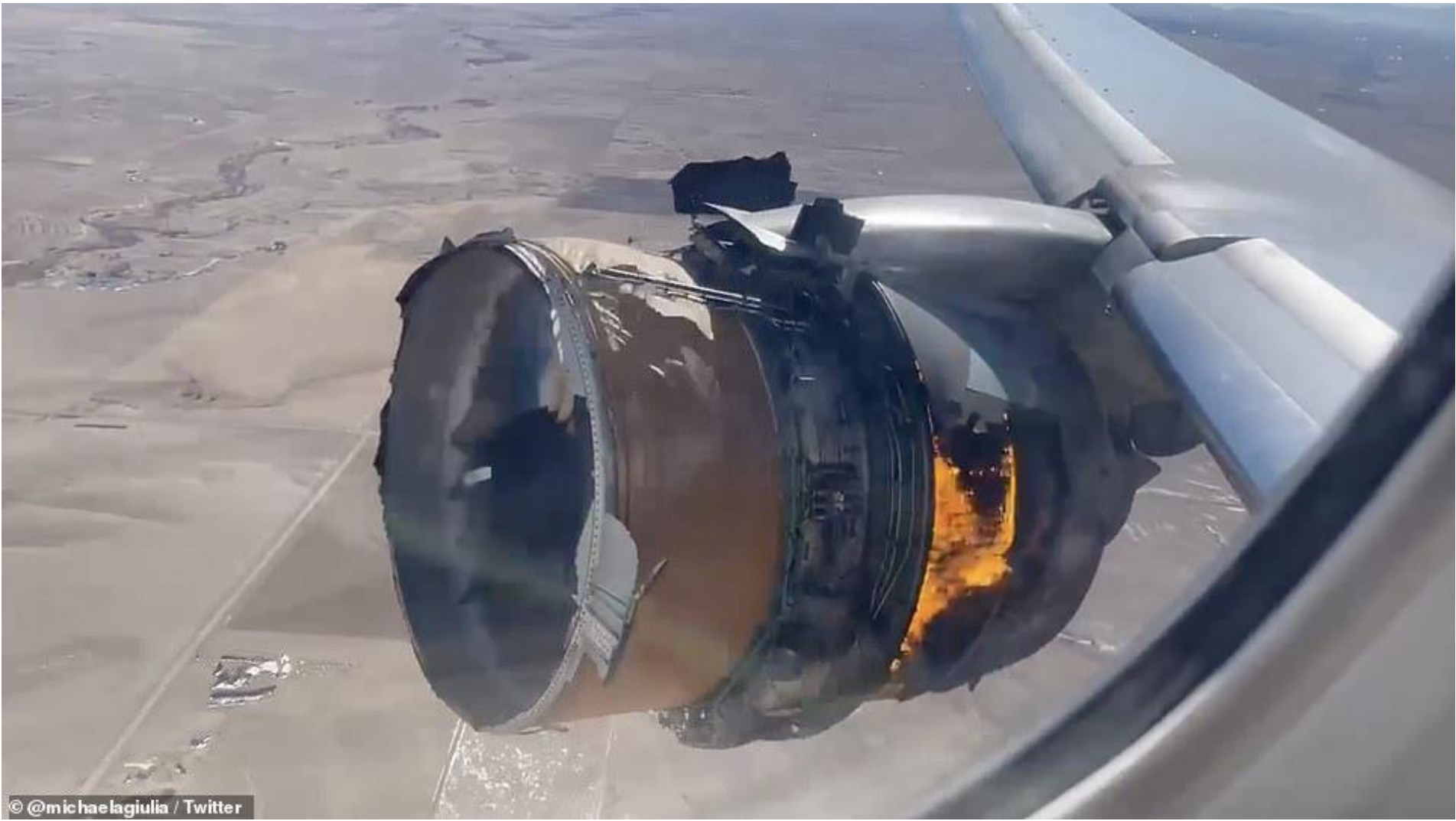
PW 4000 (777). Peso 7000kg, L=4.8m , D=2.84m , F_{max}=420kN , \alpha=6 , \pi_c=50 , Comp 1/7/11, Turb 2/7. Incidente del 20.2.2021
