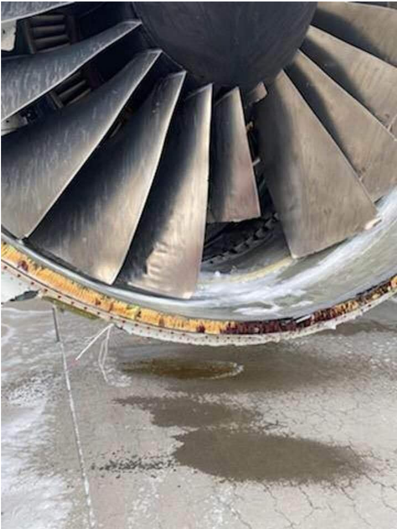
PW 4000 (777). Peso 7000kg, L=4.8m , D=2.84m , F_{max}=420kN , \alpha=6 , \pi_c=50 , Comp 1/7/11, Turb 2/7. Incidente del 20.2.2021
