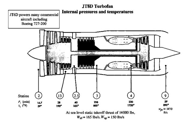
A mixed exhaust turbofan engine (JT8D from Pratt and Whitney, 1974) is described by its internal pressures and temperature, as well as air mass flow rates and the mixed jet (exhaust) velocity. Let us examine a few parameters for this engine, for a ballpark approximation.
