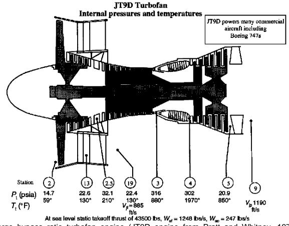
A large bypass ratio turbofan engine (JT9D engine from Pratt and Whitney, 1974) is described by its fan and core engine gas flow properties.
