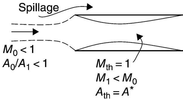
(c) At higher subsonic Mach numbers than (b) the capture ratio falls below 1 and spillage occurs (note the throat remains choked)
