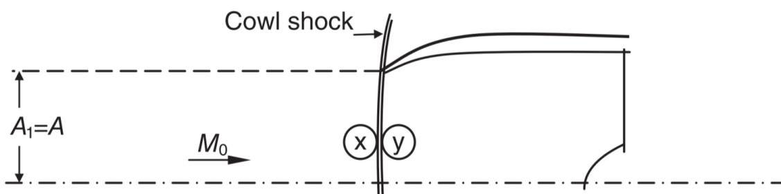
(b) Normal shock inlet in *critical mode* (low backpressure— $\dot{m}_{Design}$ )
