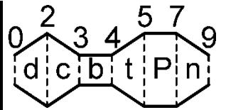
$$k = \frac{\gamma - 1}{\gamma} = \frac{0.4}{1.4} = 0.2867 \quad k_5 = \frac{\gamma_5 - 1}{\gamma_5} = \frac{0.33}{1.33} = 0.2481$$
