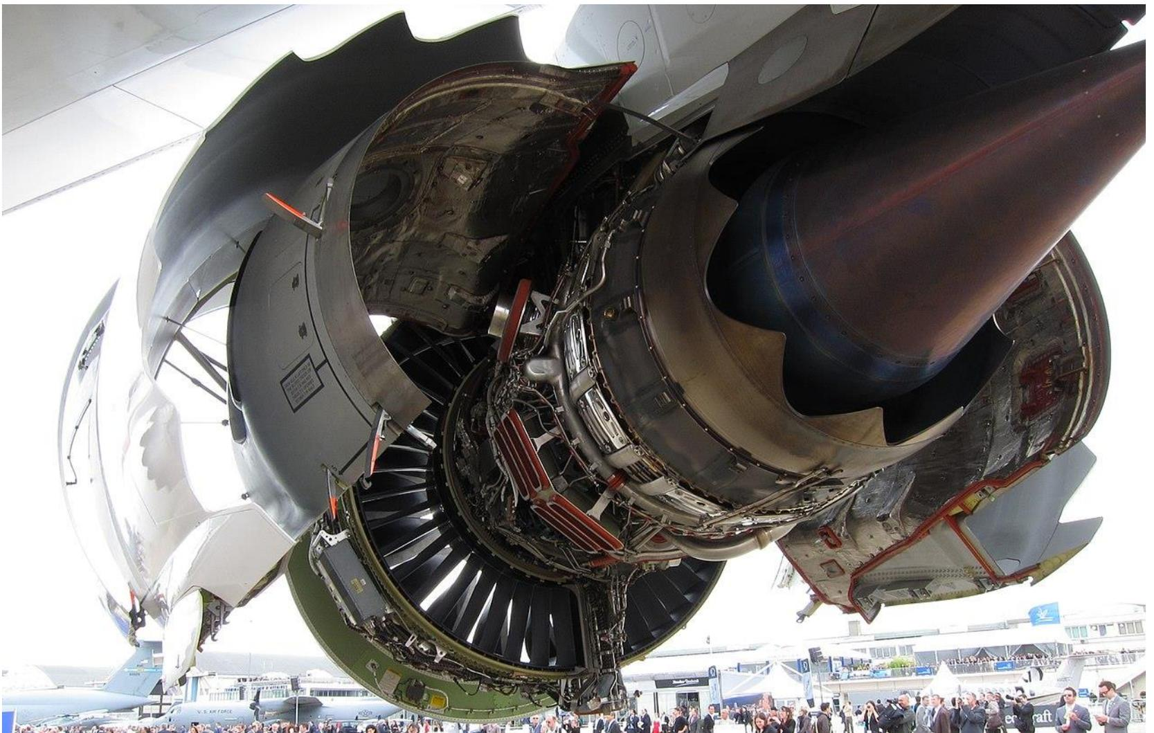
GE90 (787, 747). Peso 6150kg,  $L=4.7m$ ,  $D=2.82m$ ,  $F_{max}=330kN$ ,  $\dot{m}_a=1200kg/s$ ,  $\alpha=9.1$ ,  $\pi_c=46$ , Comp 1/4/10, Turb 2/7.
