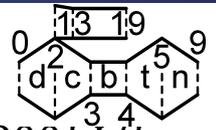
$$AB = 1, T_0 = 250K, T_{t4} = 1750K, T_{t4} = 2250, \pi_c = 26, Q_R = 42,800 \text{ kJ/kg}$$
