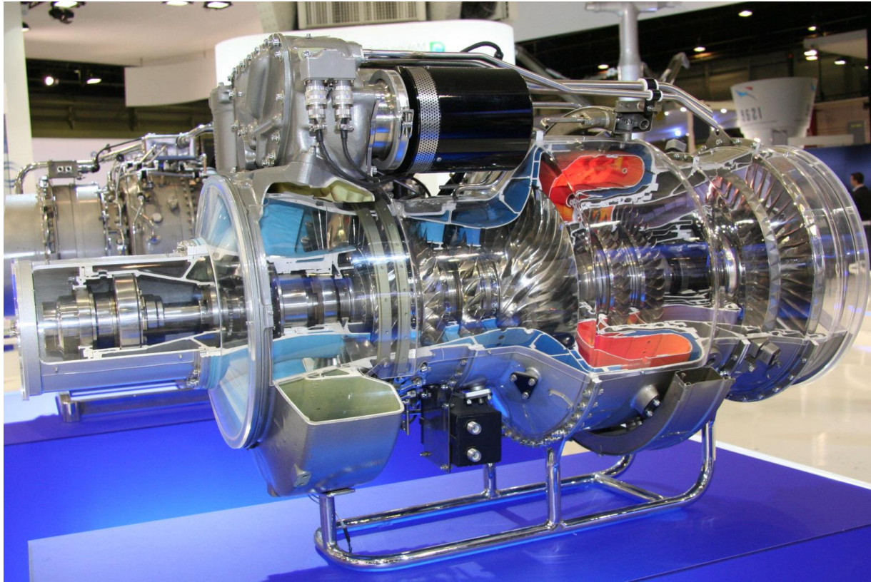
Rolls Royce turbomeca RTM322- Peso 225kg, L=1.2m , D=.65m , Equivalent Power 1700kW, Comp 3+1, Turb 2+2.
