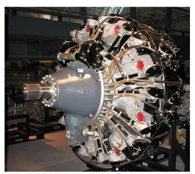
The Wright R-3350 Duplex-Cyclone is a twin-row, supercharged, aircooled, radial aircraft engine with 18 cylinders displacing nearly 55 L. Power ranged from 2,200 to over 3,700 hp (1,640 to 2,760 kW), depending on the model.
