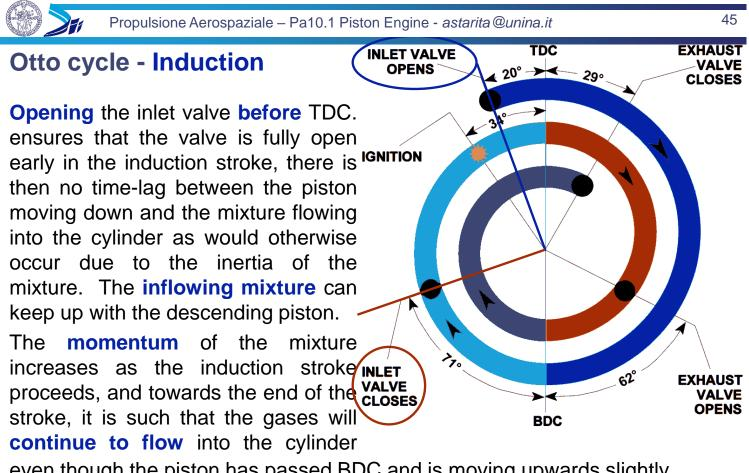
even though the piston has passed BDC and is moving upwards slightly.
