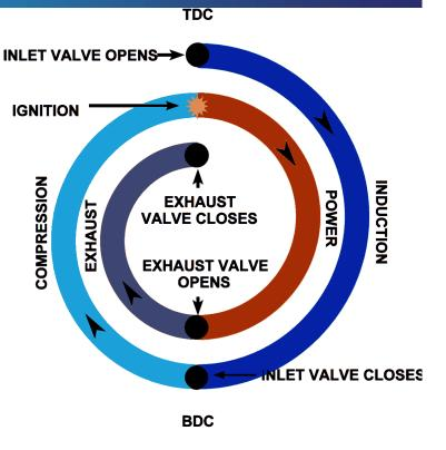
In practice the theoretical cycle proved to be inefficient and it was necessary to modify the times of valve openings and closings and ignition.
