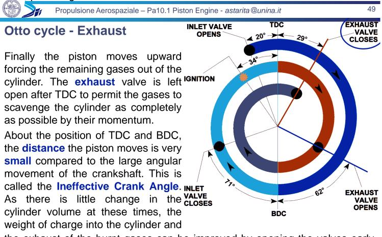
the exhaust of the burnt gases can be improved by opening the valves early and closing them late.
