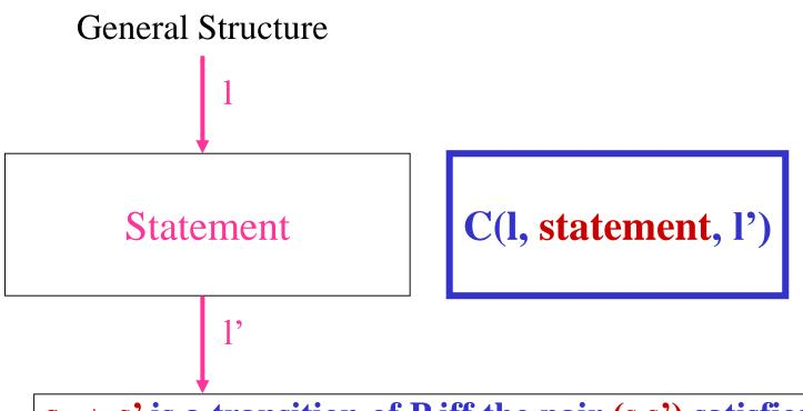
$s \rightarrow s$ ' is a transition of P iff the pair (s,s') satisfies the formula  $C(l_{init}, P, l_{end})$ , where  $l_{init}$  and  $l_{end}$  are the initial and final nodes of the CFG of P.
