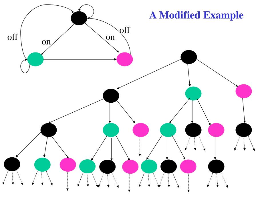
For every path  $\pi$  and every state s on that path, there is a path  $\pi$ ' starting from s and a state s' on  $\pi$ ' which is green.
