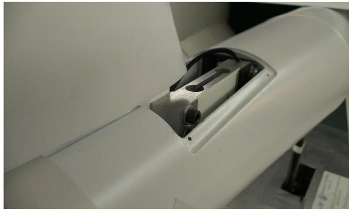
Fig 2. 13 – Vertical tail assembly with load cell
