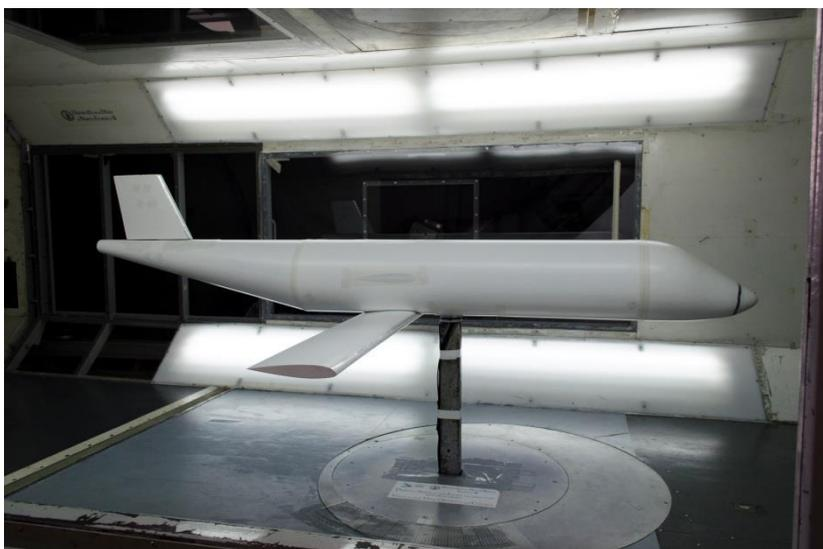
Fig 4. 26 – Example of WBV configuration with low wing
