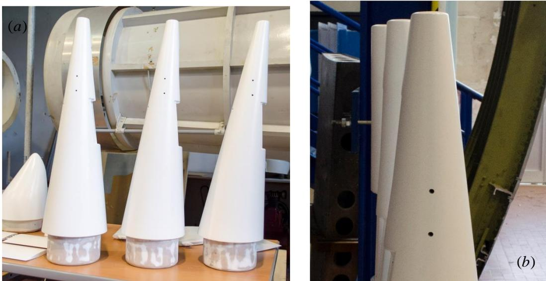
Fig 2. 11 – (a) Fuselage tail cones; (b) Sterns of the tail cones
