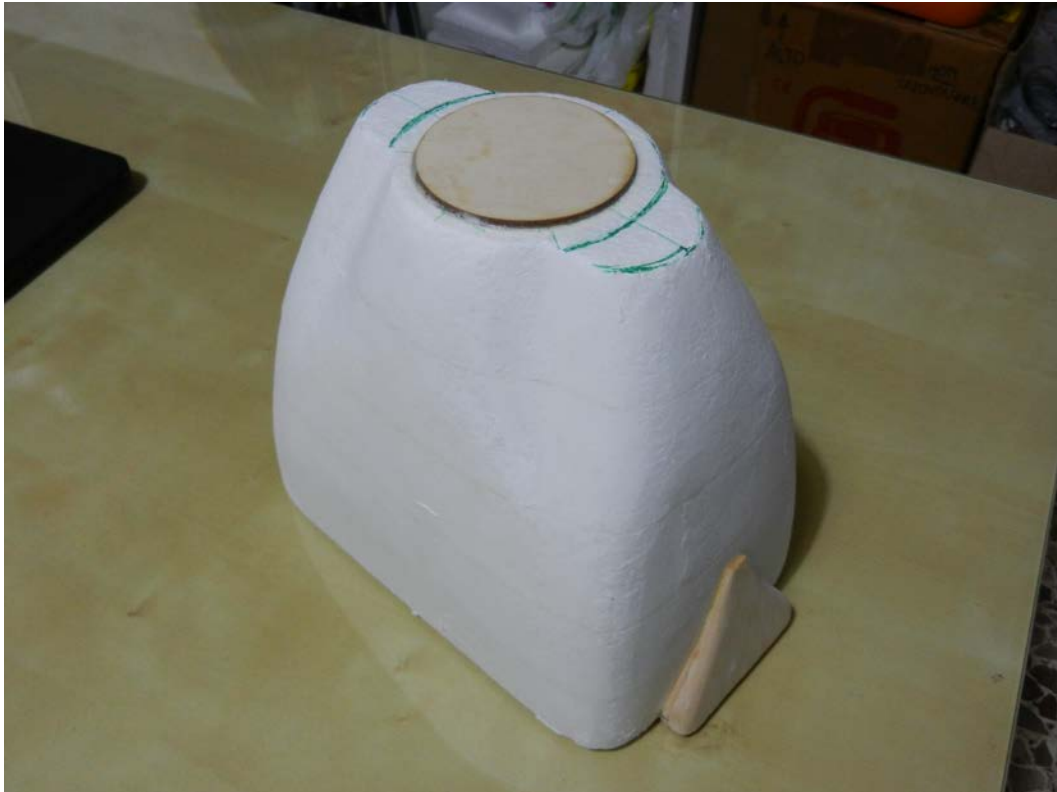
Figure 67: The shaped Styrofoam mold.
