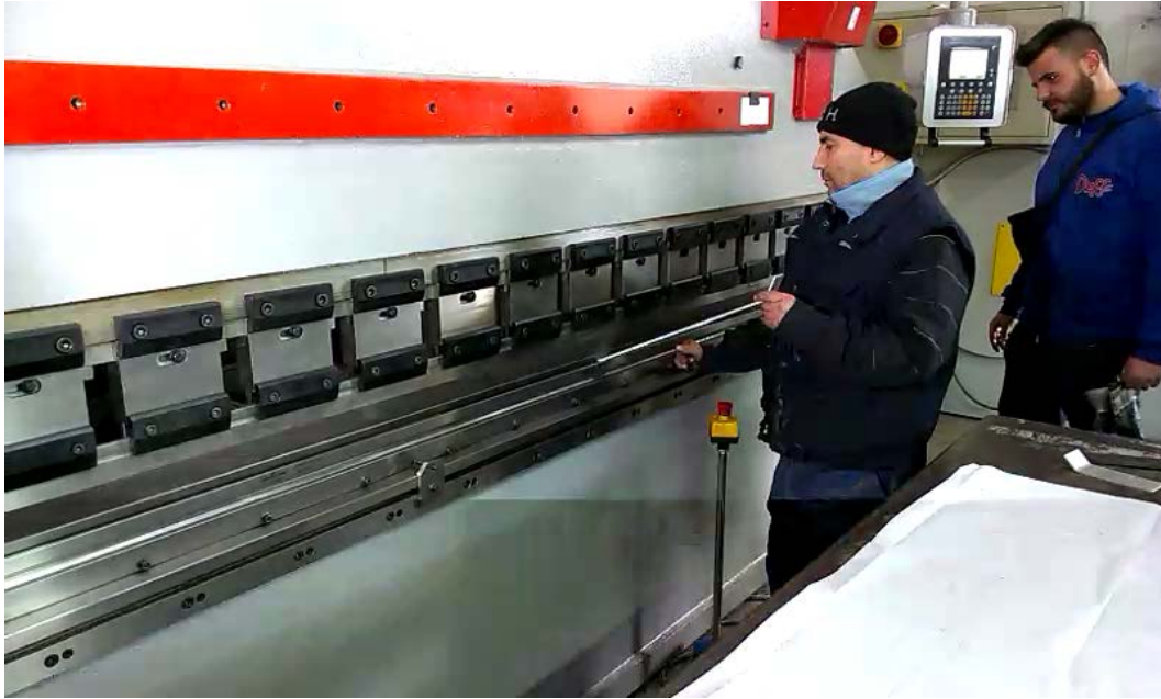
Figure 70: Bending of the landing gear plate.
