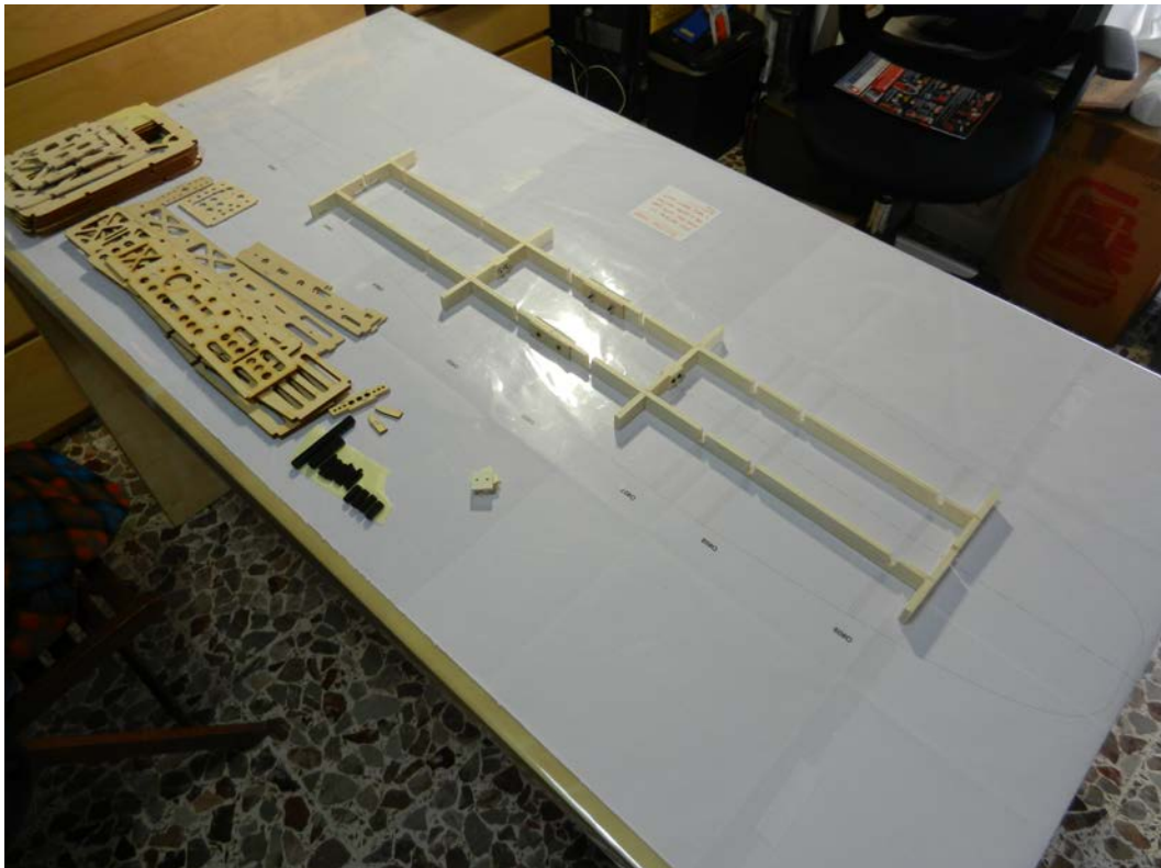
Figure 61: Fuselage assembly rail.
