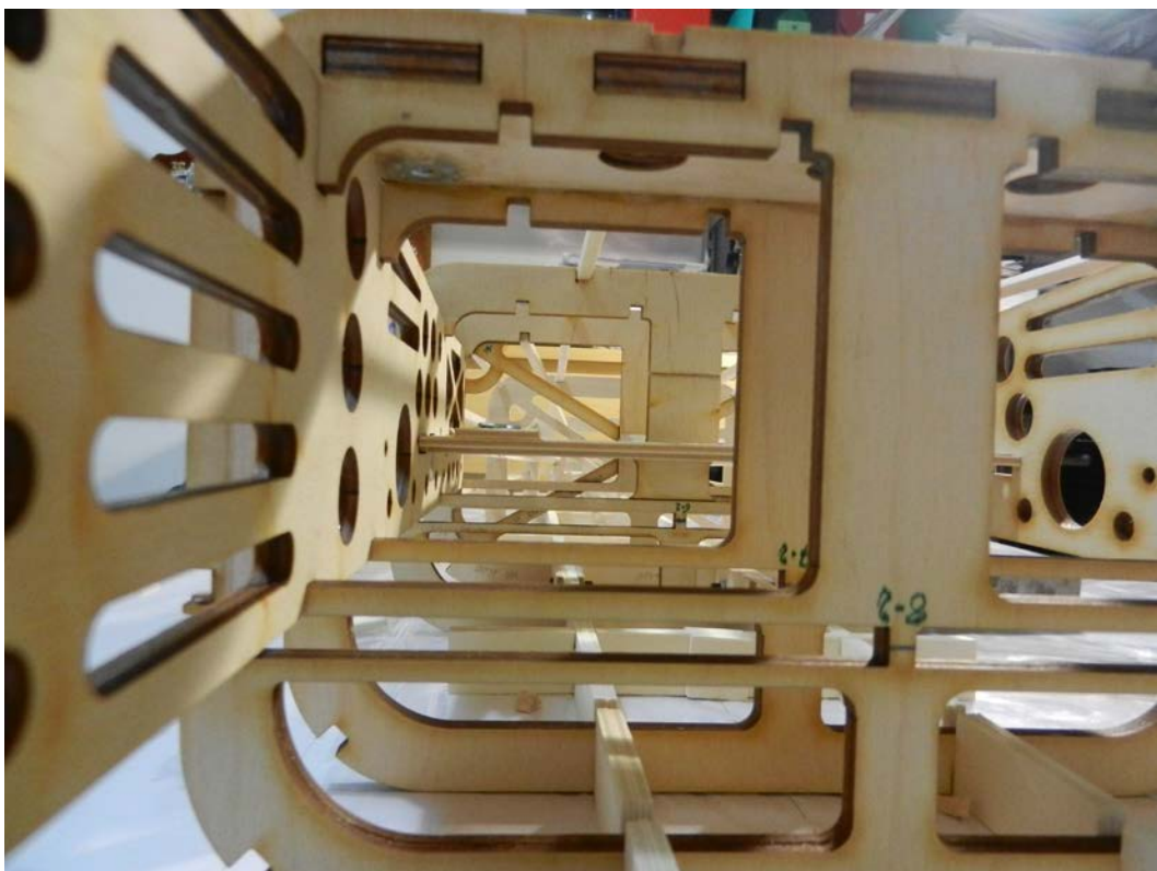
Figure 65: Precise alignment of the CNC machined parts.
