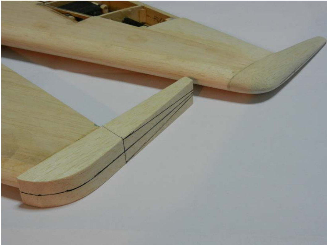
Figure 58: Comparison of tailplane tips (rough and sanded).
