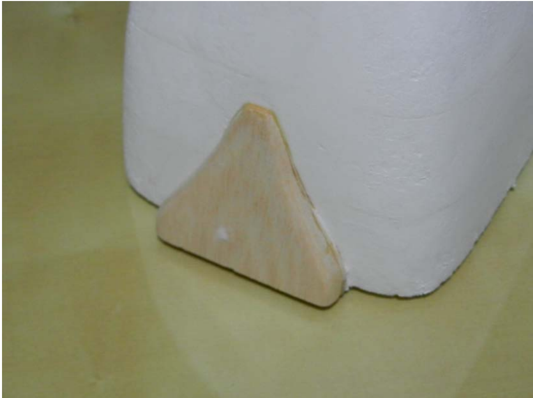
Figure 68: Cowling air outlet.
