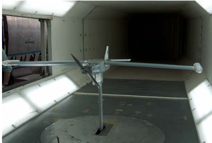
Figure 29: The reduced model in the wind tunnel.
