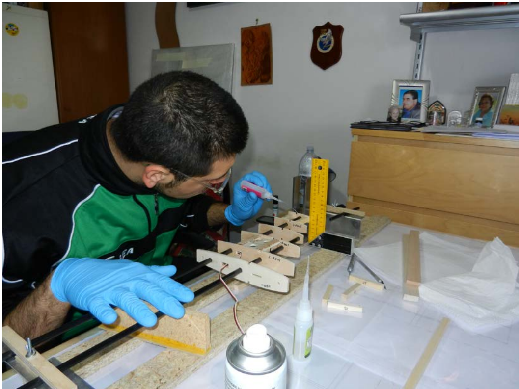
Figure 56: Assembly and bonding of the ribs.
