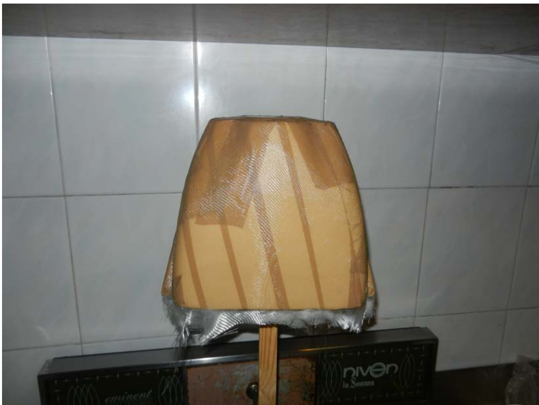
Figure 69: Fiberglass on the engine cowling.
