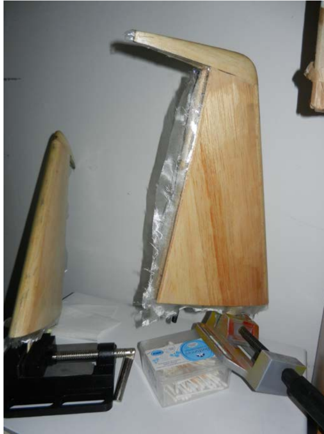
Figure 60: Tailplane covered with fiberglass.
