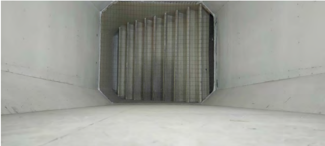
Figure 3.3 Photo of the first corner of the DII wind tunnel just located after the test section. It is easy to observe the turning vanes and the safety screen installed.
