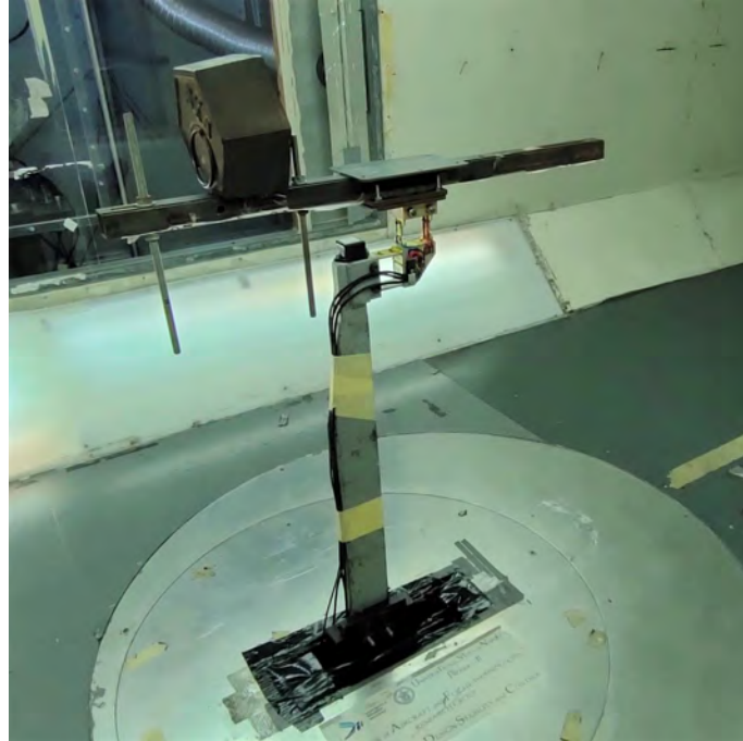
Figure 4.2 Checking the pitching moment with a 5 kg weight placed 20 cm behind the balance centre.
