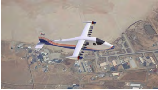
(a) NASA X-57 Maxwell: tip-mounted and leading-edge distributed propulsion.
