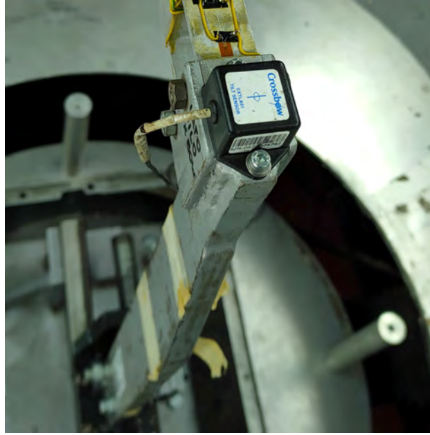
Figure 3.6 The CrossBow inclinometer mounted on the balance sting.
