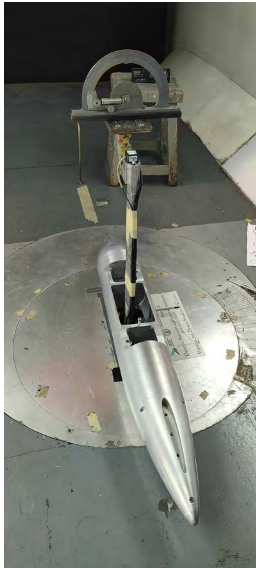
Figure 4.4 Fuselage model at the base of the sting and the level on the balance plate.
