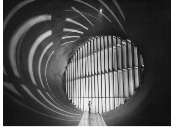
(b) The 23 vanes in the 19 foot pressure wind tunnel force the air to turn corners smoothly, https://tinyurl.com/ycxp4bny
