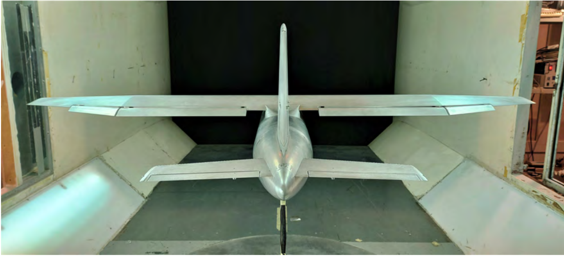
Figure 4.31 Complete aircraft model configuration with flap deflection of 15^\circ for the take-off phase.
