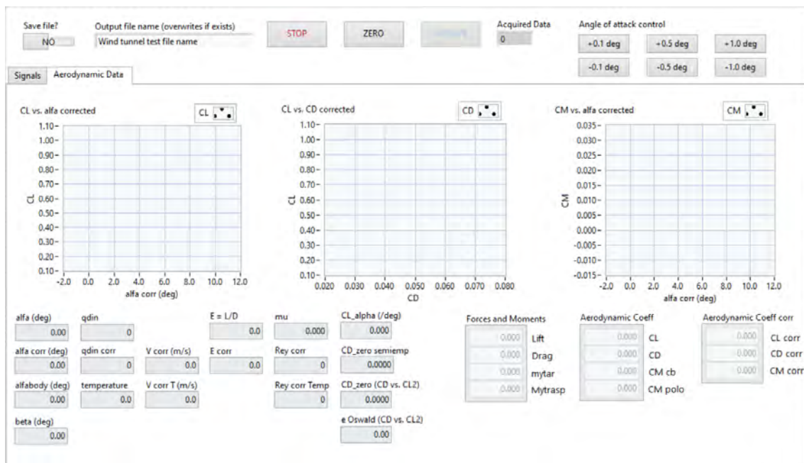
Figure 3.14 Front panel for displaying the calculated aerodynamic quantities and the acquired aerodynamic coefficients.
