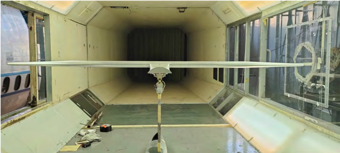
Figure 4.5 Wing installed on the balance plate.
