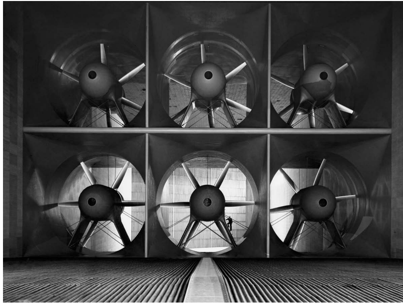
Figure 2.20 Six 40-foot diameter fans stand in the Ames 40 × 80 feet wind tunnel, https://tinyurl.com/ms8ksrw6 .
