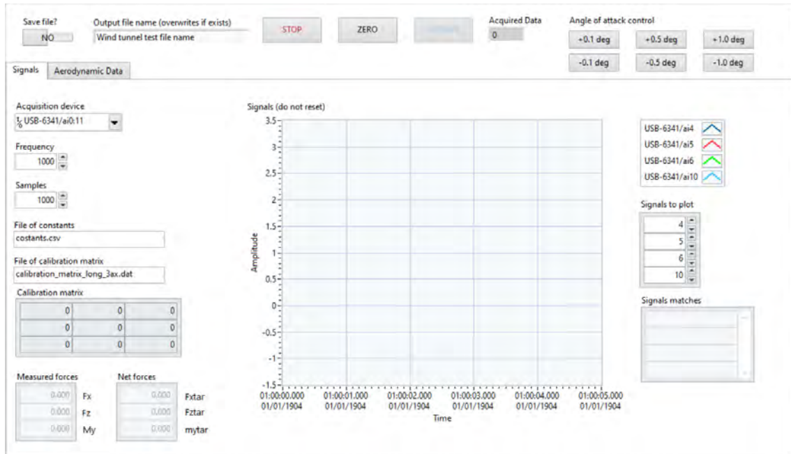
Figure 3.13 Front panel for managing the acquisition settings and displaying the acquired voltage signal.
