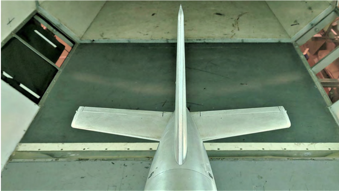
Figure 4.36 Detail of the horizontal tailpane mounted in the fuselage.
