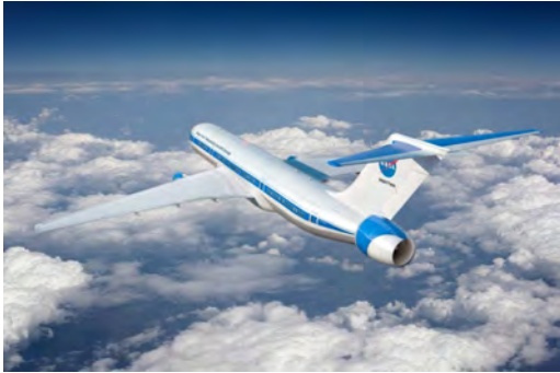
(c) NASA STARC-ABL: centerline propulsive-fuselage concept with boundary-layer ingestion.
