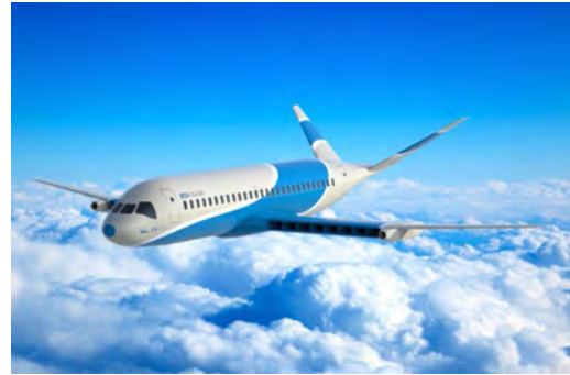
(d) ESAero ECO-150: concept with two turbo-electric generator and sixteen electric ducted fans.
