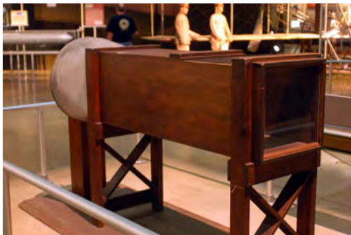
(a) Wright brothers 1901 replica of wind tunnel. National Museum of the United States Air Force. https://tinyurl.com/mr287fwz
