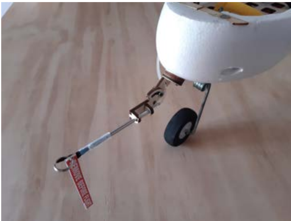
Figure 4.15: Pitot tube installed on the nose of the aircraft
