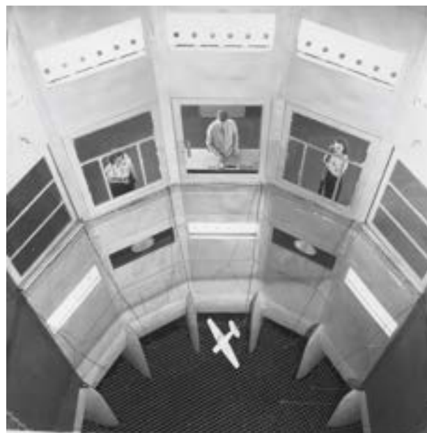
Figure 1.3: Test section of the 20-foot spin tunnel at Langley Research Center [4]
