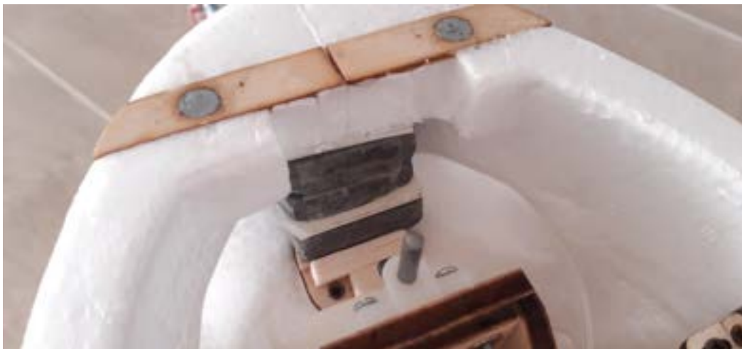
Figure 4.22: Sky Hunter ballast weight made up by lead bricks
