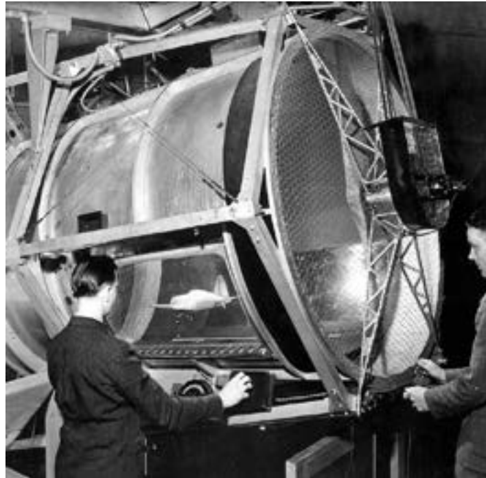
Figure 1.4: Free-flight test of an aircraft model in a free-flight tunnel [4]
