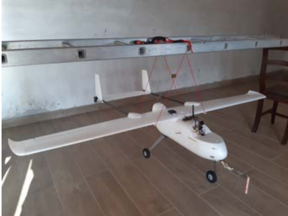
Figure 4.23: Roll moment of inertia test bench - Sky Hunter
