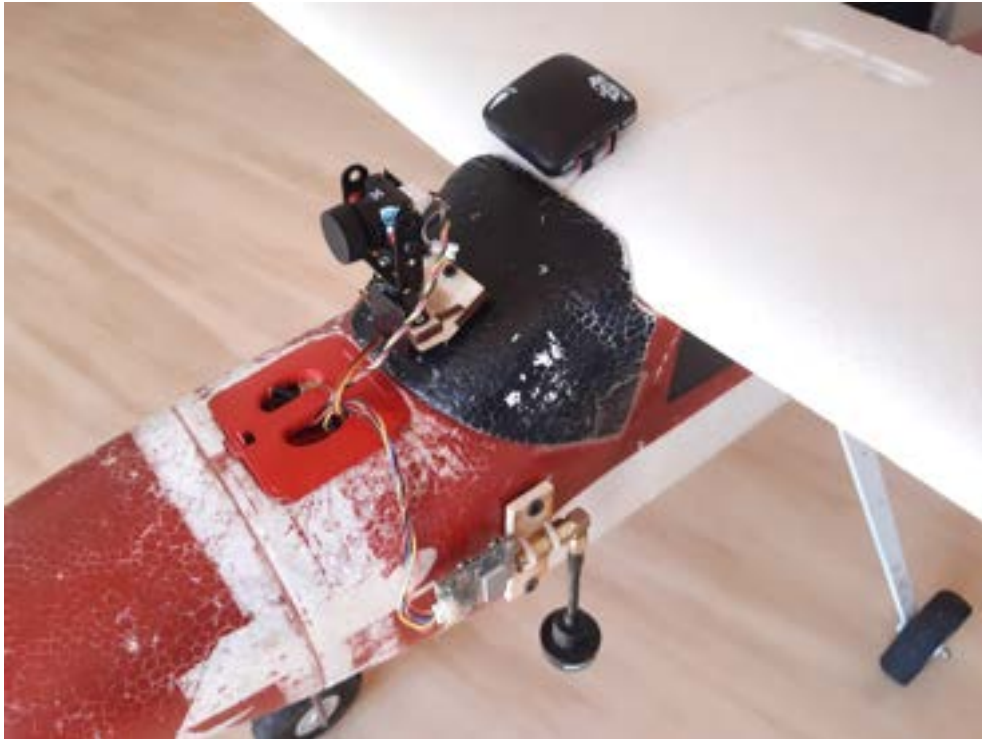
Figure 3.7: GPS and FPV System installed on the U CAN FLY
