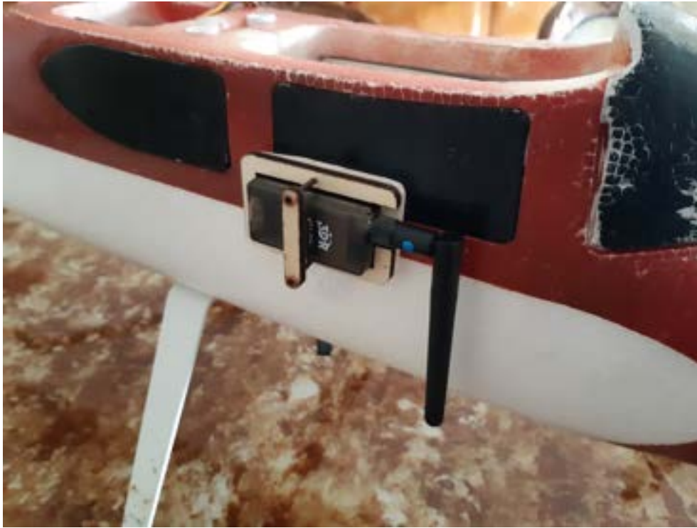
Figure 3.6: Telemetry radio installed on the U CAN FLY
