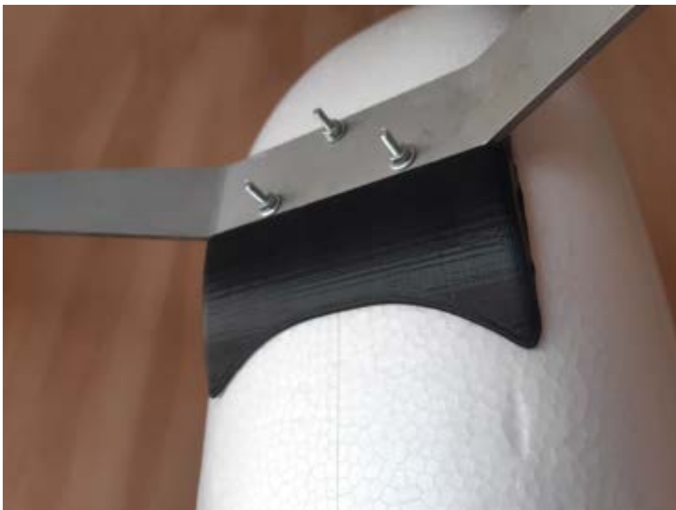
Figure 4.4: Main gear 3D printed fairing - Sky Hunter
