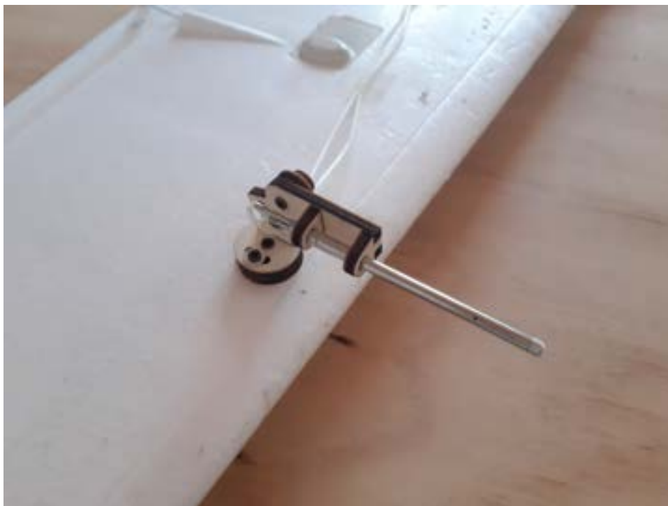
Figure 3.5: Underwing Pitot mount - U CAN FLY
