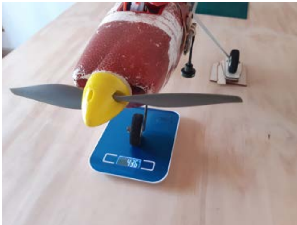
Figure 3.19: Nose gear load measurement - U CAN FLY
