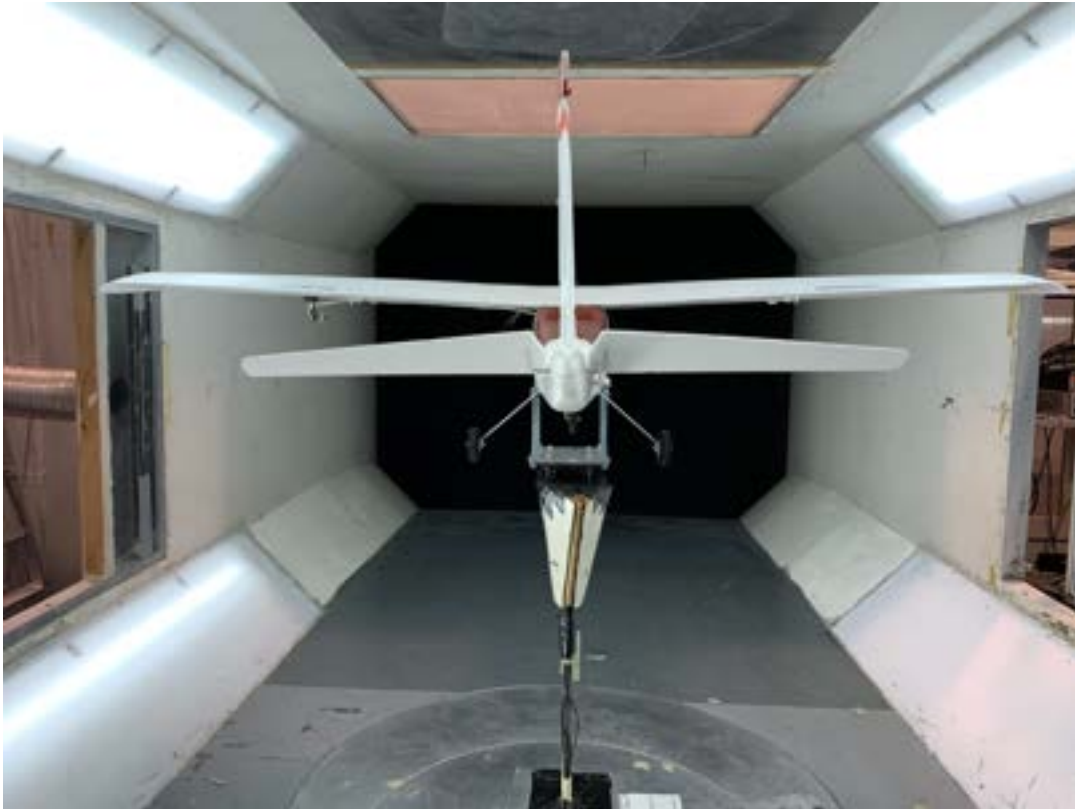
Figure 3.36: Back view of U CAN FLY highlighting the elevator deflection
