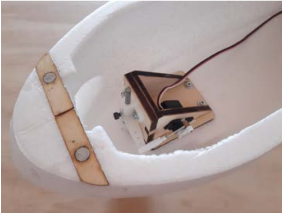
Figure 4.6: Nose gear mount bolted to the fuselage - Sky Hunter
