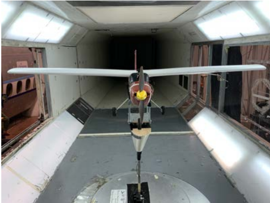
Figure 3.30: Front view of U CAN FLY mounted in wind tunnel
