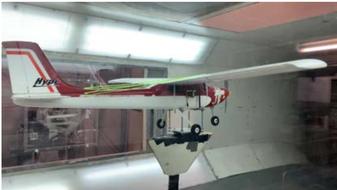
Figure 3.35: U CAN FLY wind tunnel test. Thin strings attached to the wing to highlight the airflow around it
