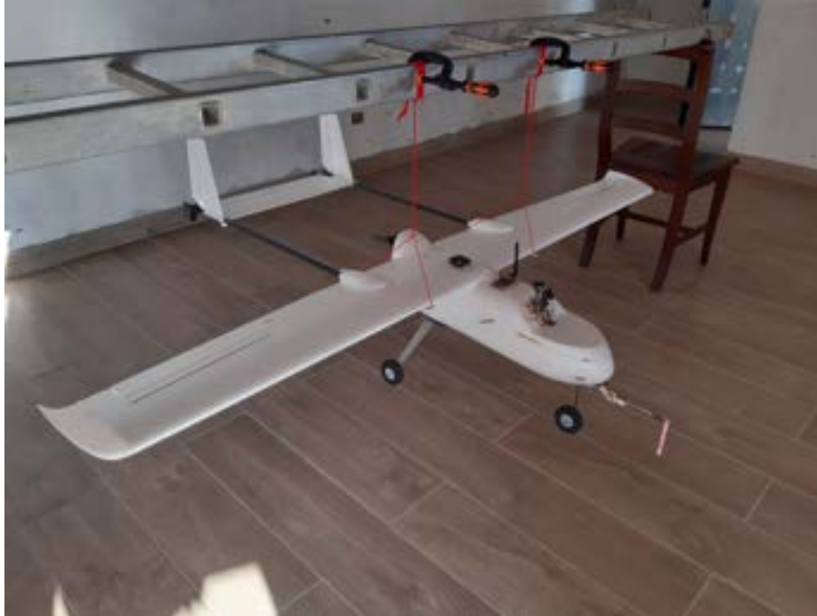
Figure 4.27: Yaw moment of inertia test bench - Sky Hunter
