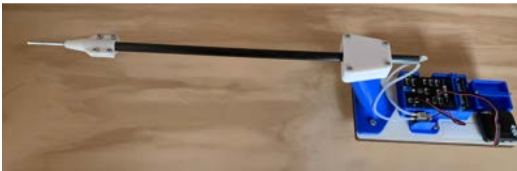
Figure 3.14: Airspeed sensor mount for wind tunnel testing
