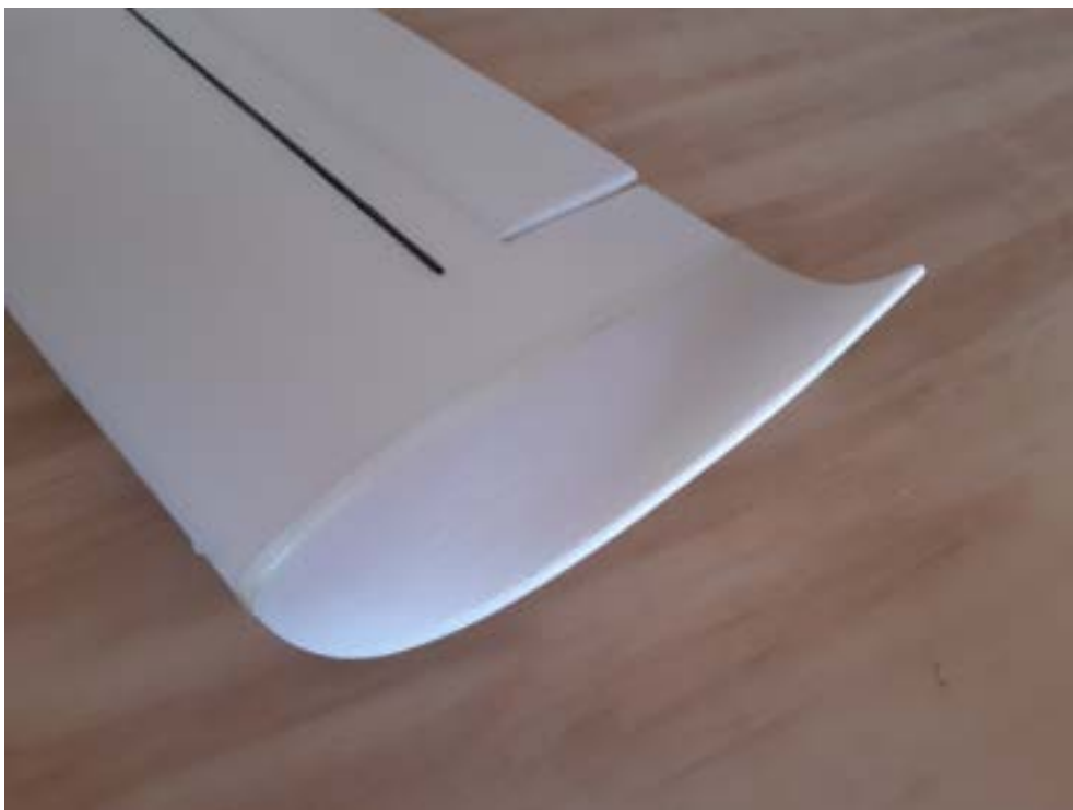
Figure 4.11: 3D printed wingtip bolted to the tip mount - Sky Hunter
