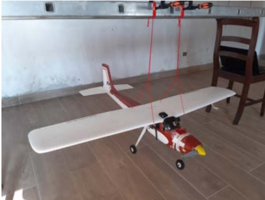
Figure 3.25: Yaw moment of inertia test bench - U CAN FLY
