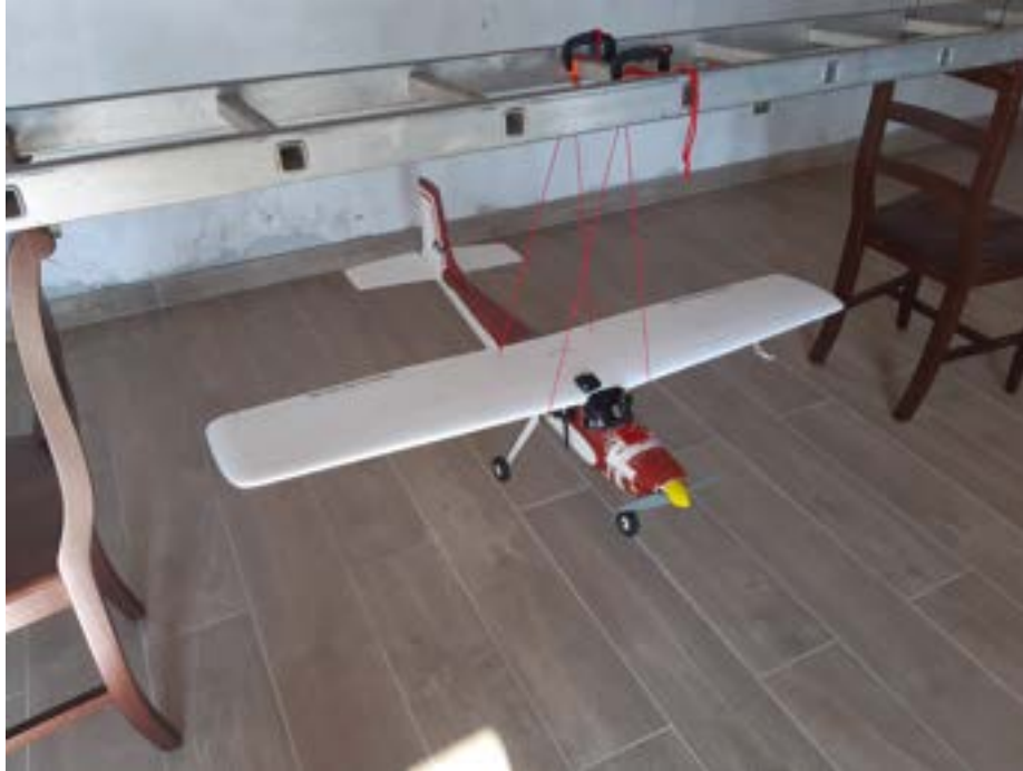
Figure 3.21: Roll moment of inertia test bench - U CAN FLY
