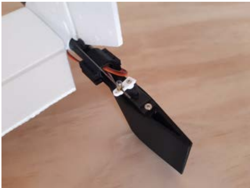
Figure 4.8: Servo mount detail - Sky Hunter
