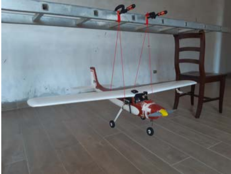
Figure 3.23: Pitch moment of inertia test bench - U CAN FLY
