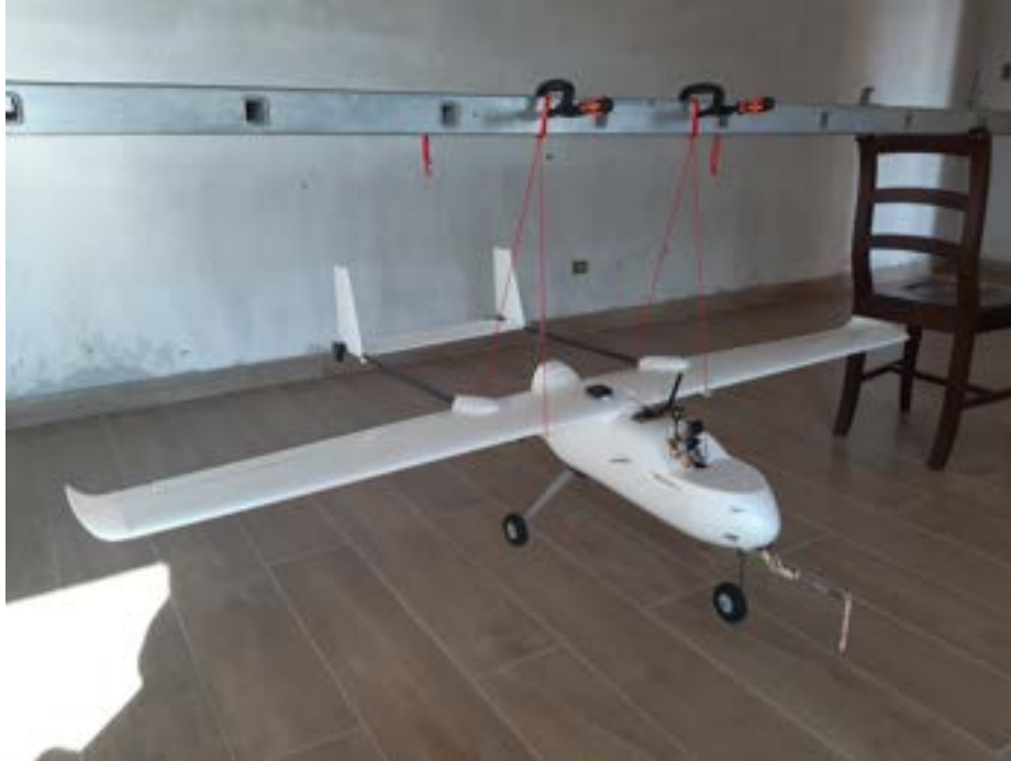
Figure 4.25: Pitch moment of inertia test bench - Sky Hunter
