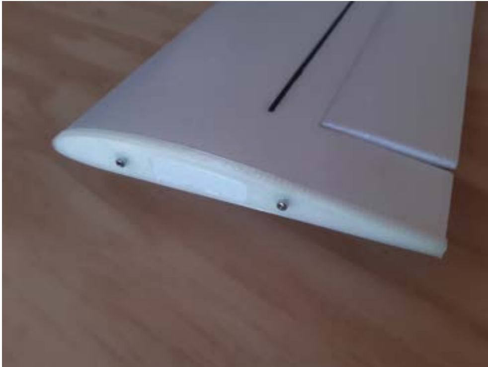
Figure 4.10: 3D printed tip mount - Sky Hunter
