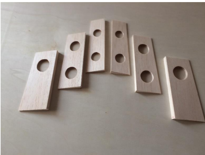
Figure 22: The six sections ready to be glued to the leading edges.
