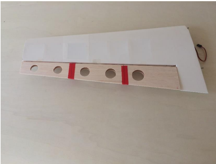
Figure 27: Semi-completed wing, with uncovered ailerons and temporary tape stripes.
