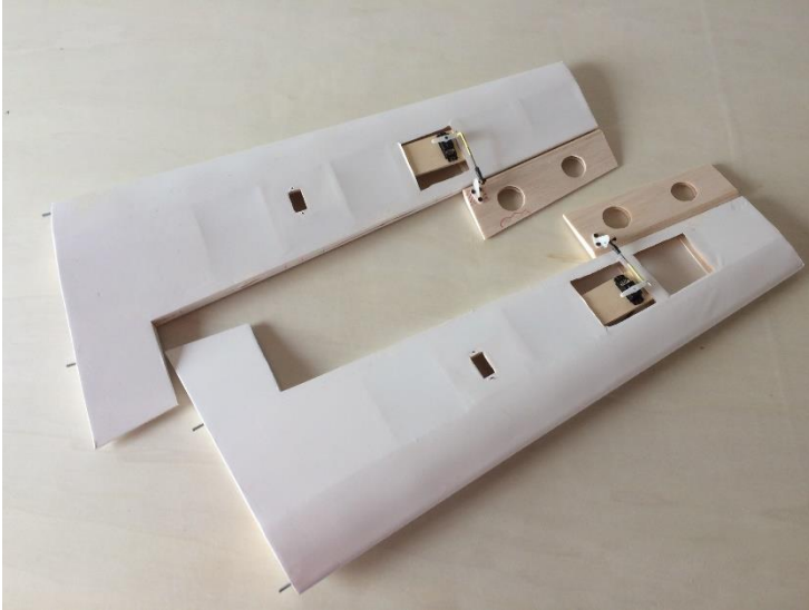
Figure 26: A new servo plywood base was mounted on the wing, closer to the wingtip, in order to move the external section of the aileron. The original servo mounting holes were covered with tape.
