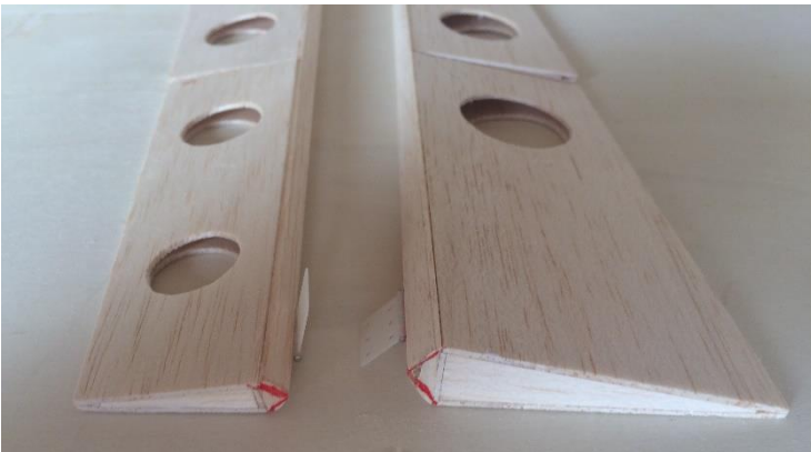
Figure 24: The ailerons after sanding, the LEs shape allows a maximum deflection of about 40 degrees.
