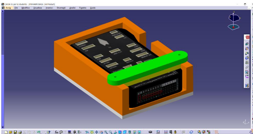
Figure 40: PIXHAWK housing in the CATIA™ Design Environment. The balsa parts are colored in orange, the Depron® base is white. A 4 mm plywood locking bar (colored in green) is screwed to the balsa frame.
