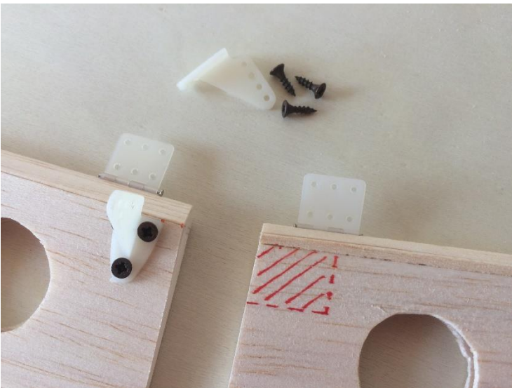
Figure 25: Each external section was reinforced with a 4 mm plywood base, glued under the balsa skin, in order to place a nylon control horn locked by self-tapping screws.
