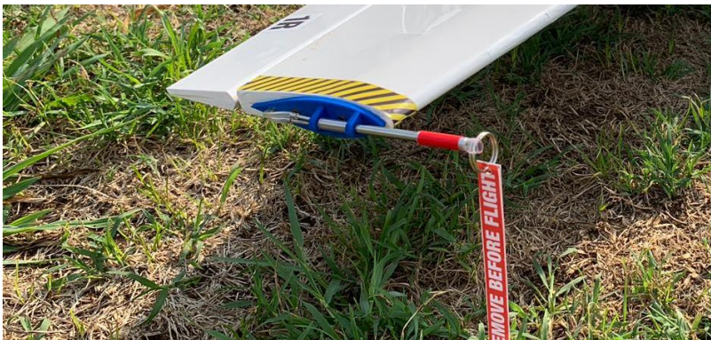
Figure 43: Pitot tube installed and connected to the pressure sensor. The wingtip was highlighted with a striped tape and a silicone tube with a safety message was used for protecting the Pitot holes from any kind of dust.
