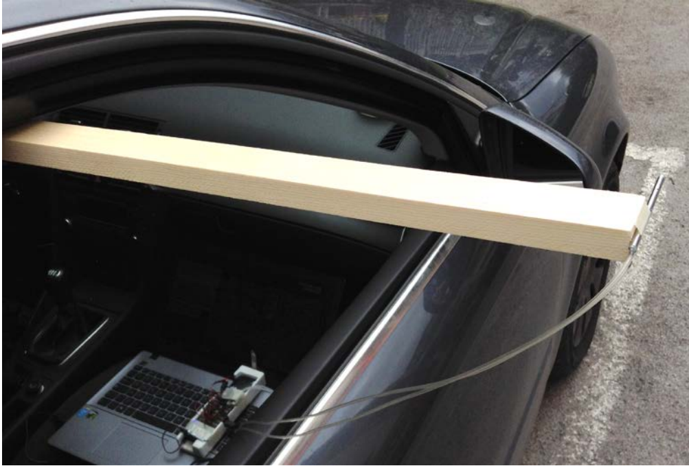
Figure 19 : Airspeed sensor calibration verification test set-up
