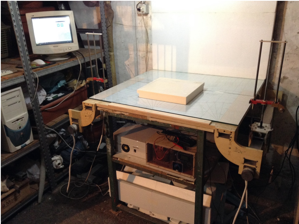
Figure 29 : CNC hot wire foam cutting machine
