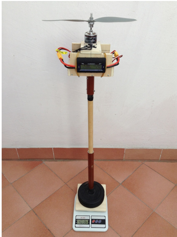
Figure 13 : Static thrust test rig
