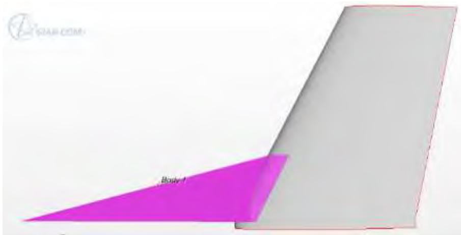
Figure 25 – The Final Reference Geometry of Dorsal fin.
