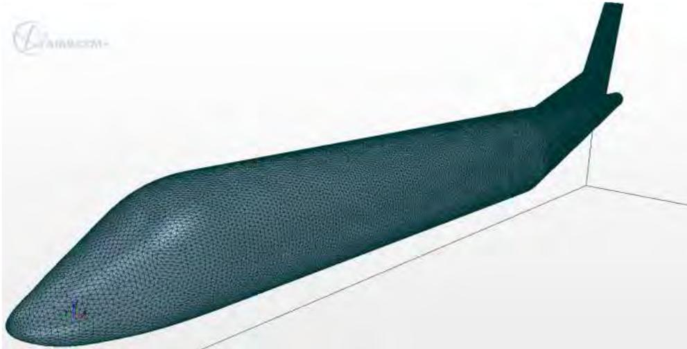
*Figure 51 – Tetrahedral Mesh Surface of STAR-CCM+.*
