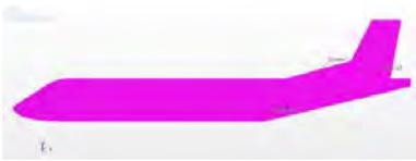
For BVD we obtain the same shape of VD but with a reduction of stability due to the fuselage negative contribution. Also in this case after  $\beta=19^\circ$  the slope increase, so we can attribute this effect at the dorsal fin presence.
