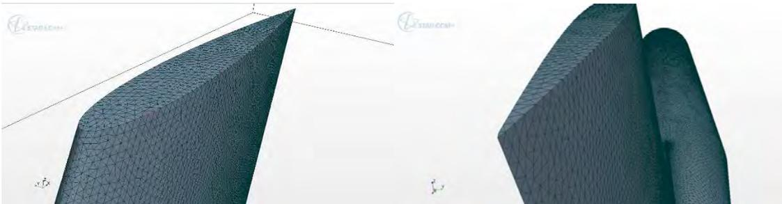
**Figure 64 – Sharp edges of the vertical edges of the tip section and the trailing edge.**
