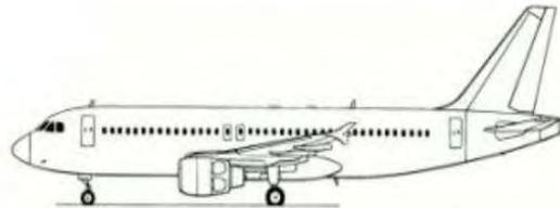
**Figure 42 – View and side view of a round edge dorsal fin of an A 320 (Prendrel 2013 and Aerospaceweb 2013).**
