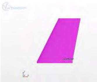
For the V we obtain an angle-of-stall about  $\beta=19^\circ$ , then there are a quite constant value until  $\beta = 26^\circ$ , after we can see an increase of yawing moment due to the low AR which characterize this particular geometry. The actual stall is reached at  $\beta = 38^\circ$ .
