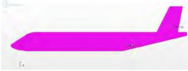
For BV we obtain the same shape of V but with a reduction of stability due to the fuselage negative contribution. Also in this case there is a first negative variation of slope about  $\beta=19^\circ$  related to the vertical stall, then after  $\beta=26^\circ$  there are an increases of slope until  $\beta=40^\circ$ .
