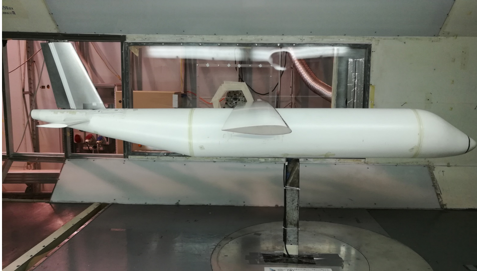
Figure 4.3 Assembly B with an aspect ratio of 1.5, body tail cone high, wing high, body-mounted horizontal tail. Re = 470000 , \alpha = 0^\circ
