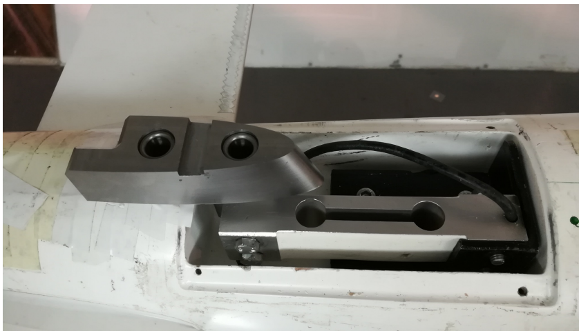
Figure 2.6 The common base of the vertical tail assemblies mounted on the off-center load cell.
