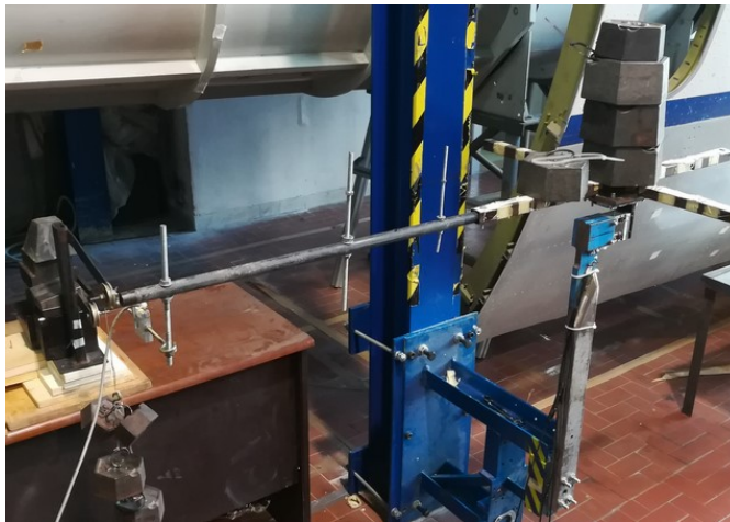
Figure 3.4 Verification of the internal strain gage balance.
