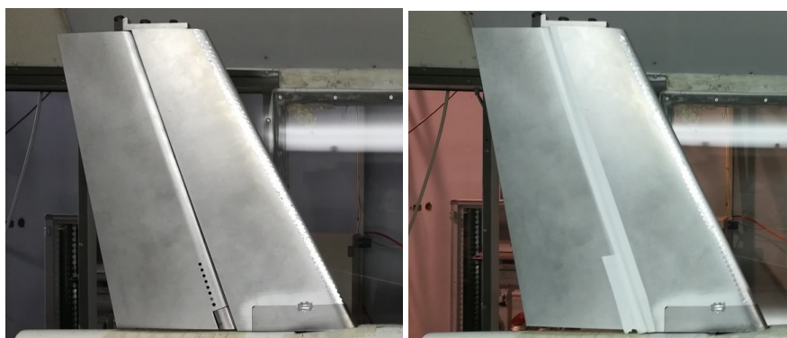
Figure 3.8 The tail assembly A involved in the investigation about the effects of the rudder gap. Re = 470\ 000 , \beta = 0 deg.
