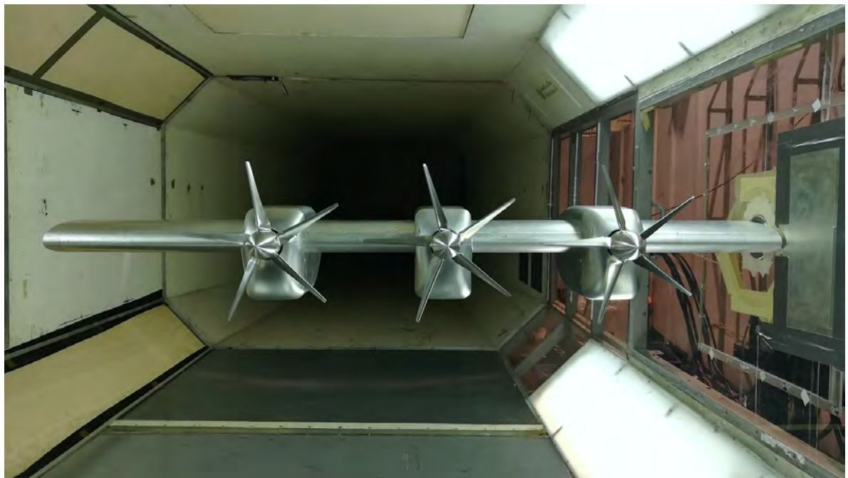
Figure 4.2 – DEP prop-on configuration
