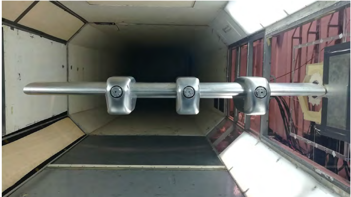
Figure 4.1 – DEP prop-off configuration
