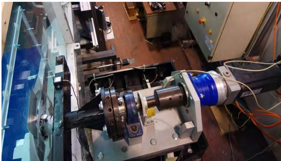
(b) The electric motor above the wind tunnel balance
