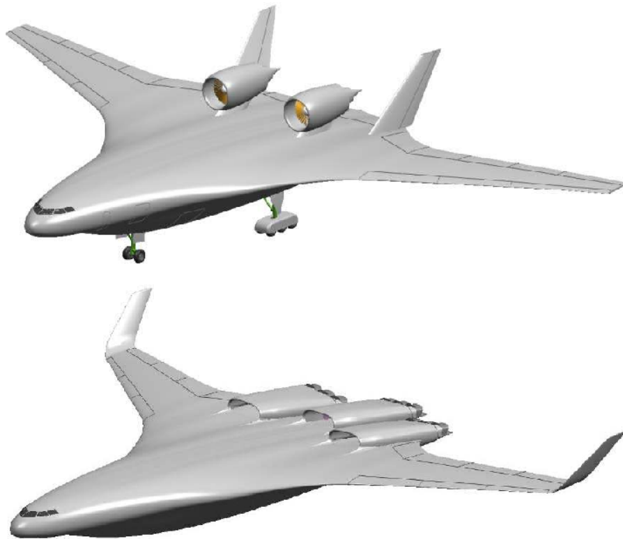
Figure 1.10: Example of a podded and embedded with distributed propulsion engine for a BWB aircraft.
