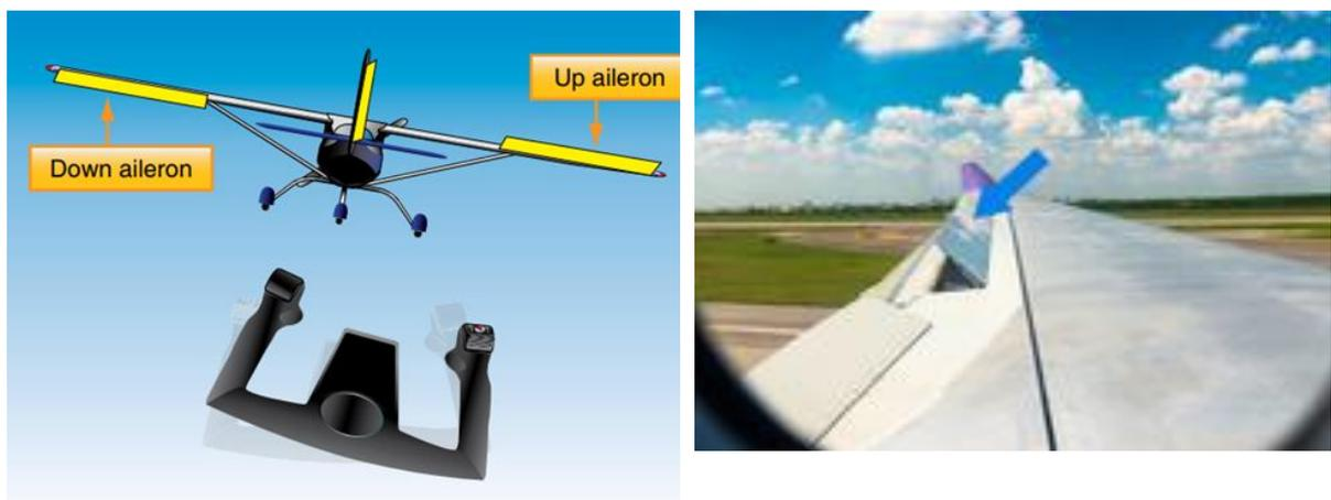
**Figure 2.4 – Ailerons operation.**
