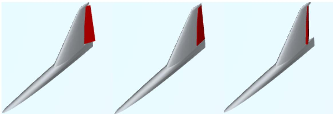
*Figure 3.14 – C-130 Hercules rudder operation ( $-30^\circ$ ,  $0^\circ$ ,  $+30^\circ$ ).*
