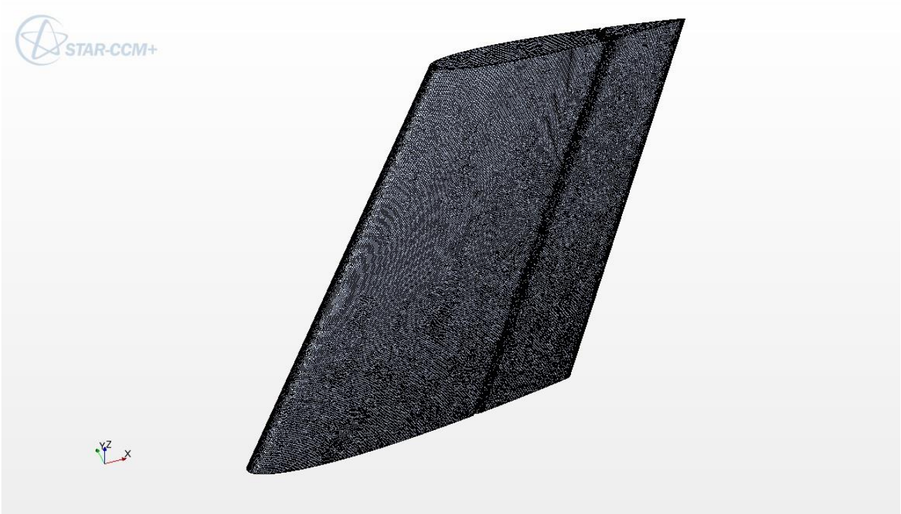
Figure 73: Computational grid for Geometry 1, \delta_r = 0^\circ .
