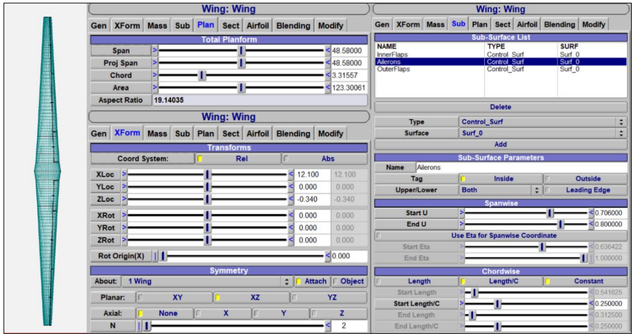
Figure 3.6 – Some parameters of the wing and ailerons
