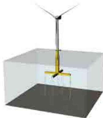
Qualification of innovative floating substructures for 10MW wind turbines and water depths greater than 50m.
