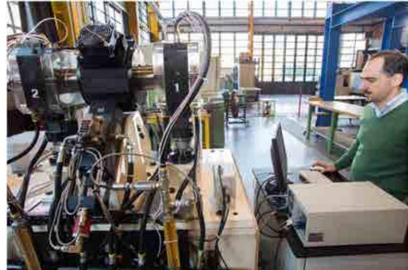
Tilting-pad journal brg.  $\phi 100$  mm, 25 kN, 3000 rpm
