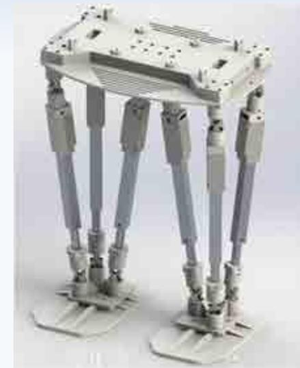
**A prototype of the proposed Cassino biped locomotor for experimental tests**
