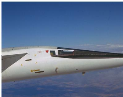
(a) *Nose Up*
