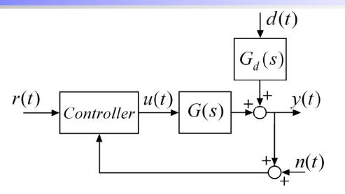
The objective of a control system is to make the output of a plant y(t) behaving in a desired way, by manipulating the plant input u(t)
