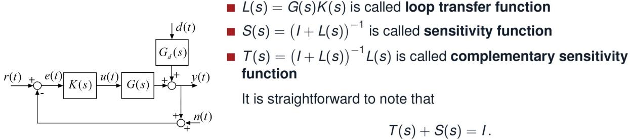
Exploiting the composition rules for block diagrams, it turns out that
