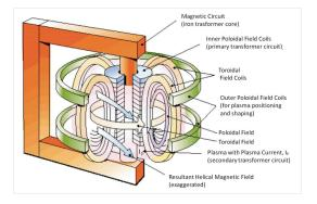
A tokamak is an electromagnetic machine containing a fully ionised gas (plasma) at about 100 million degrees within a torus shaped vacuum vessel. Poloidal and toroidal field coils, together with the plasma current, generate a spiralling magnetic field that confines the plasma.
