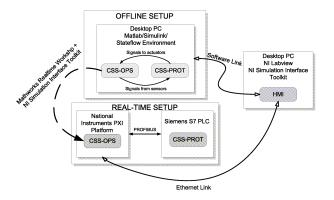
By using automatic code generation (ACG) tools, the control system prototype and the plant simulator are deployed on real-time targets, in order to validate the real implementation of the safety control system by means of HIL simulations.
