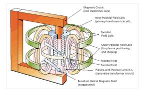
A tokamak is an electromagnetic machine containing a fully ionised gas (plasma) at about 100 million degrees within a torus shaped vacuum vessel. Poloidal and toroidal field coils, together with the plasma current, generate a spiralling magnetic field that confines the plasma. A flexible architecture for the rapid prototyping of control systems in fusion experiments
