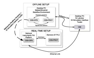
architecture for the rapid prototyping of control systems in fusion experiments
