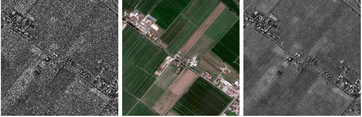
Fig. 1. A single-look SAR image, a co-registered optical image, and the SAR image despeckled based on a multitemporal data.
